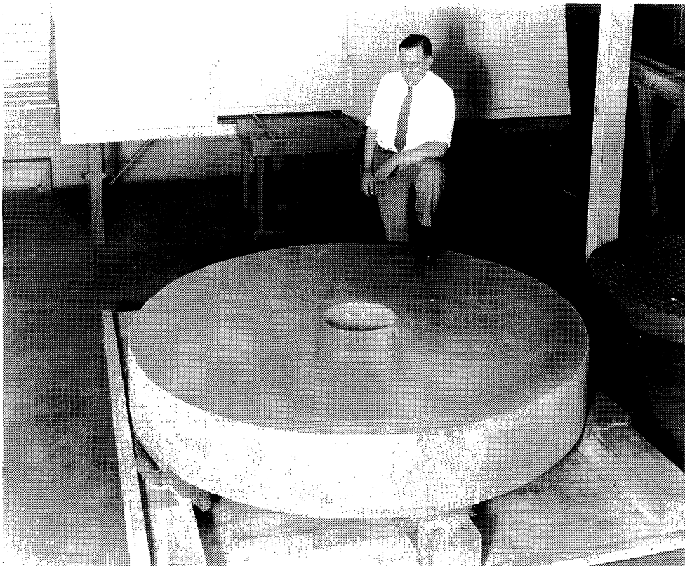
Figure 3. Robert Lundin in the Warner & Swasey optical shop, with the recently-delivered glass blank for the 82-inch McDonald Observatory reflector, 1934 © Astral Press • Provided by the NASA Astrophysics Data System
