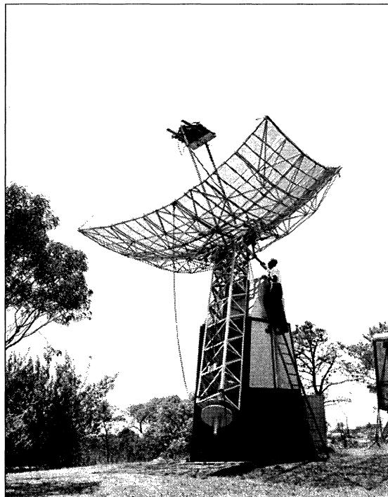
Figure 4: The 16 x 18-ft paraboloid on a polar mount. Jim Hindman, on the top of the ladder, was involved in both solar and H-line observations (courtesy ATNF Historic Photographic Archive: B2649-2).
