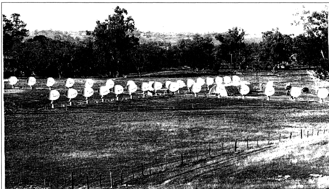
Figure 1: The 9.2 cm spectroheliograph.
