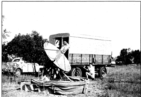
Figure 30: The 1.1 metre dish at Potts Hill, used by Minnett and Labrum for solar observations at 9,428 MHz. Norman Labrum is crouching beside the old mobile instrument trailer (ATNF Historic Photographic Archive: B1581-2).
