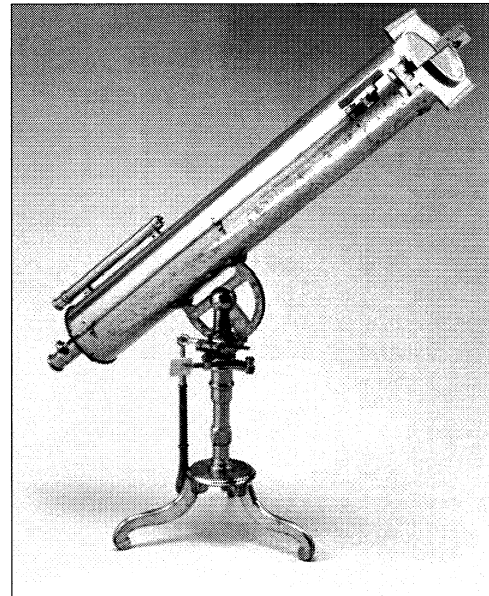
Figure 12: Two foot Gregorian telescope and stand by Sir James Short, with split-lens micrometer, ca.1763. Made for the Royal Society of London for the observation of the 1769 transit of Venus.
