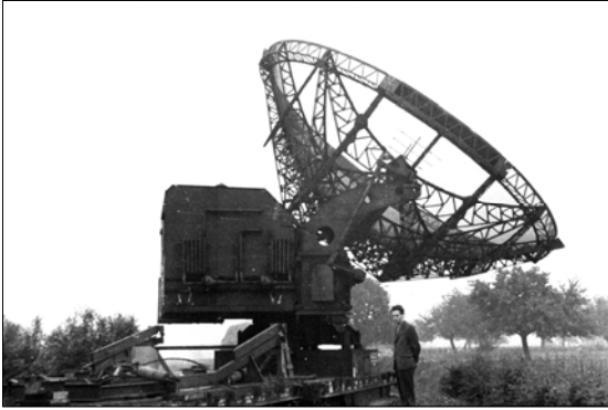
Figure 2: The 7.5m Würzburg antenna at Marcoussis used for the solar eclipse observations (courtesy: Observatoire de Paris, Meudon).
