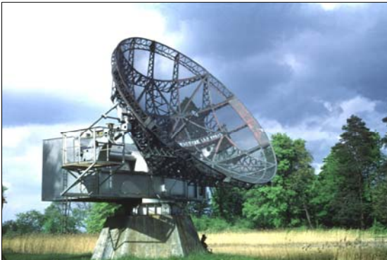
Figure 3: The 7.5m Würzburg antenna at Meudon used for the solar eclipse observations (courtesy: Observatoire de Paris, Meudon).
