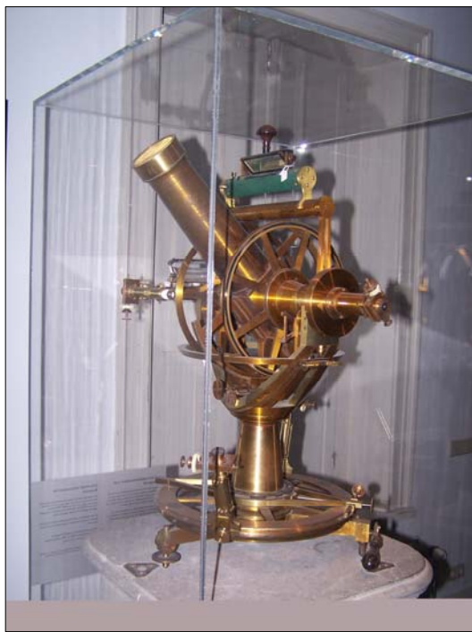
Figure 8: The Repsold universal instrument at the Utrecht Observatory (courtesy: Dr Roland Wittje).
