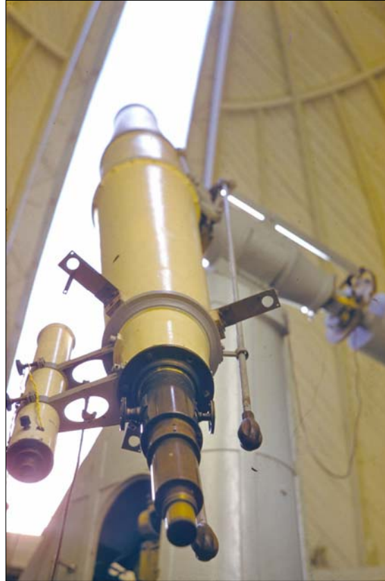
Figure 4: The 11.75-inch refractor at Dunsink Observatory, known as the 'South Telescope' after Sir James South who in 1863 presented the lens, made by Cauchoix of Paris in 1829, to Dublin University. It was installed by Thomas Grubb of Dublin in 1868, and was a favourite instrument of Robert Ball. It is still in place. When it was made, the lens was the largest object glass in existence and was used in 1830 by Sir John Herschel to discover the sixth star in the Trapezium in the Orion Nebula. This photograph was taken in the 1950s by Hermann Brück (courtesy of Mary Brück).
