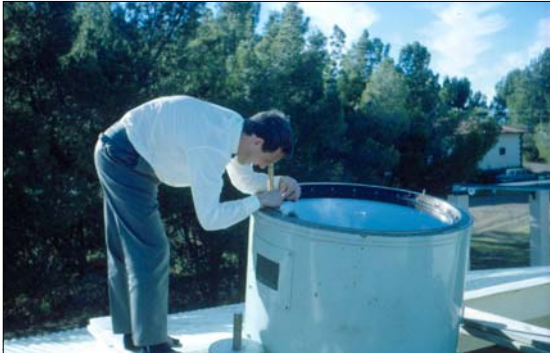
Figure 5: David Andrews using the small centering telescope to check the alignment of the ADH Telescope in 1966 (photograph supplied by the author).
