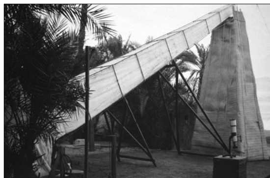
Figure 10: The 40-foot Schaeberle Camera on the bank of the Nile in Egypt (Mary Lea Shane Archives).
