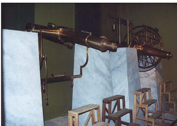
Figure 10: The Reichenbach and Ertel transit telescope (foreground) and meridian circle (background) of the 1820s, now on display in the 'New Meridian Room' at the Observatory (photograph by the author).
