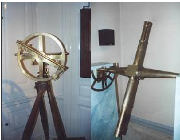
Figure 7: Period instruments at the Stockholm Observatory. On the left is the geographical circle by Daniel Ekström (near his original workroom) and on the right an eighteenth century transit instrument located in the ‘Old Meridian Room’ (photographs by the author).
