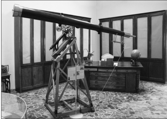
Figure 9: The Steinheil telescope following restoration work, on the wooden mount that was made by ARASS (Association for the Restoration of Ancient Scientific Instruments) of Milan, which also made the hour and declination circles. In the background, the large desk that was used by Guido Horn d'Arturo, to whom the room in which the telescope is exhibited is dedicated (courtesy: Museo della Specola, University of Bologna).
