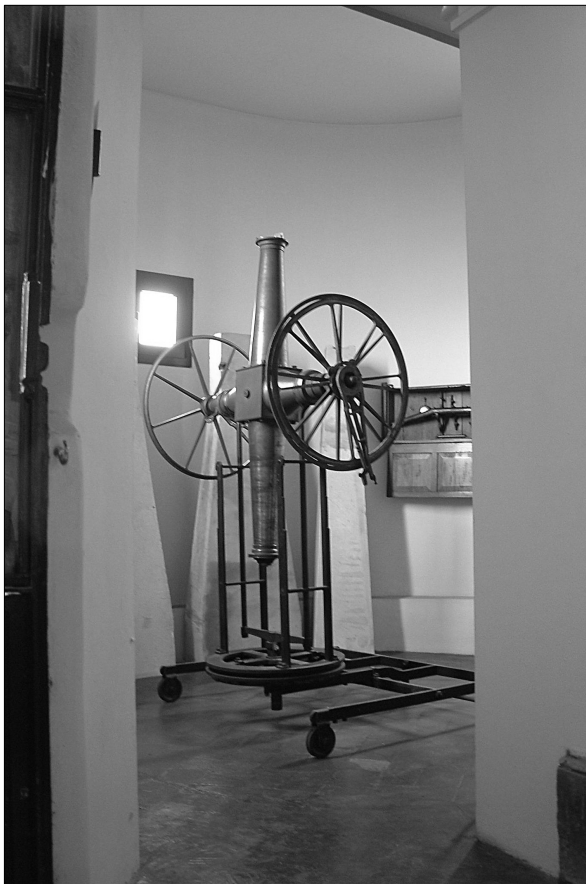
Figure 3: What remains today of the Ertel & Sohn meridian circle, repositioned in its original dome. One of the pillars is visible in the background (courtesy: Museo della Specola, University of Bologna).
