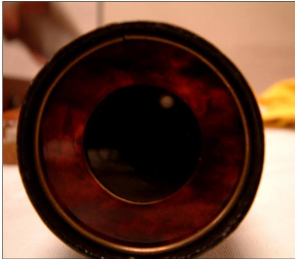
Figure 2a (above): The objective lens with a tortoiseshell aperture stop.
