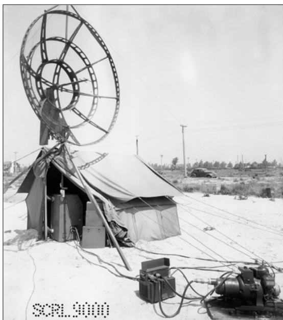
Figure 4: An AN/TPS-3 radar in operation in 1944 (courtesy CE LCMS Historical Office Department of the Army, USA).
