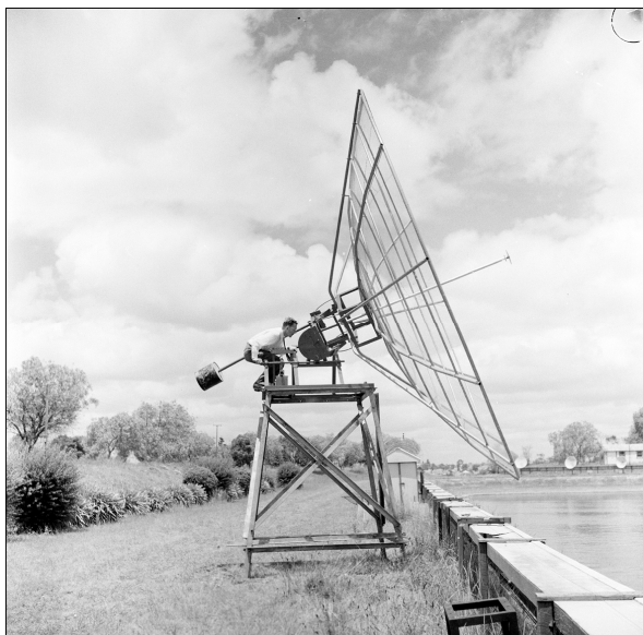
Figure 23: Close-up of the 5.8m Fleurs Chris Cross prototype antenna undergoing testing at Potts Hill (courtesy ATNF Historical Photographic Archive).
