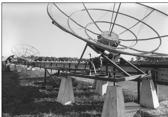
Figure 9: Close up of the north-south grating array, looking south, showing the robust equatorial mounting and the use of mesh rather than a solid reflector (courtesy ATNF Historic Photographic Archive).
