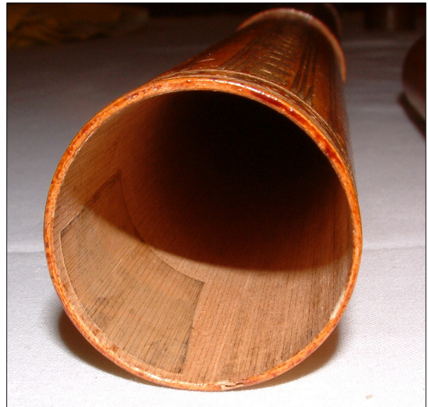
Figure 3a (left): The surface decoration of the telescopic tube. Figure 3b (above): The inside view of the tube made of thin wooden sheets.
