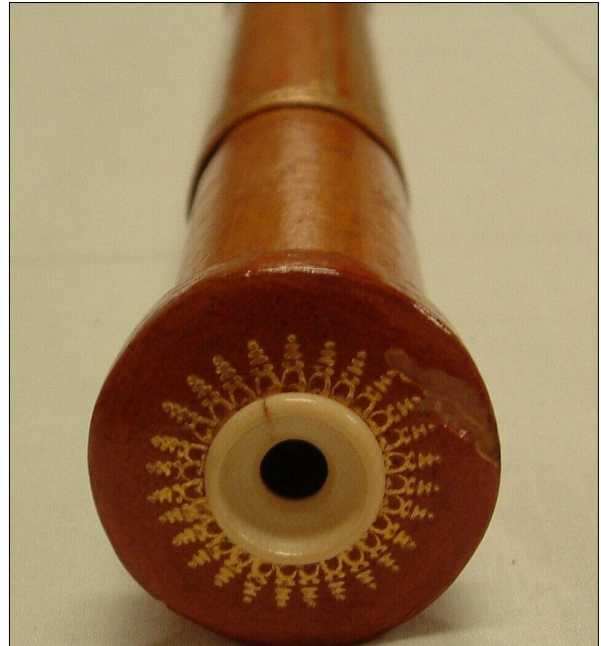
Figure 2a (above): The objective lens with a tortoiseshell aperture stop.
