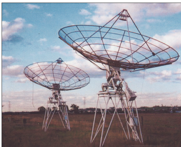
Figure 53: Leon Darcy's 2-element interferometer at Bungonia, which utilises two ex-Chris Cross antennas and mountings (courtesy Don Whiteman).
