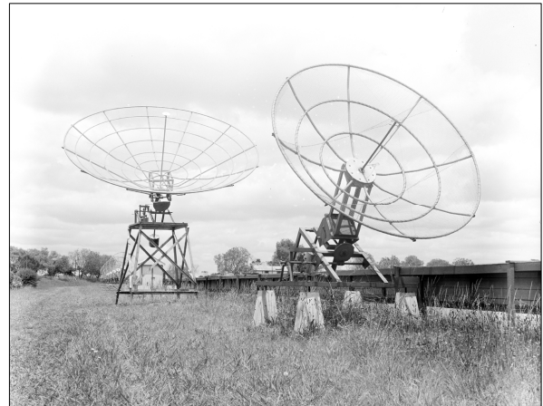
Figure 9: The Chris Cross test antenna at Potts Hill (second from right), shown between elements in the N-S grating array (courtesy ATNF Historic Photographic Archive: B3881-2).
