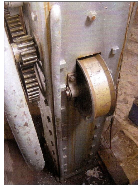
Figure 11: The Edinburgh guide wheel (courtesy: Allan Marshall).
