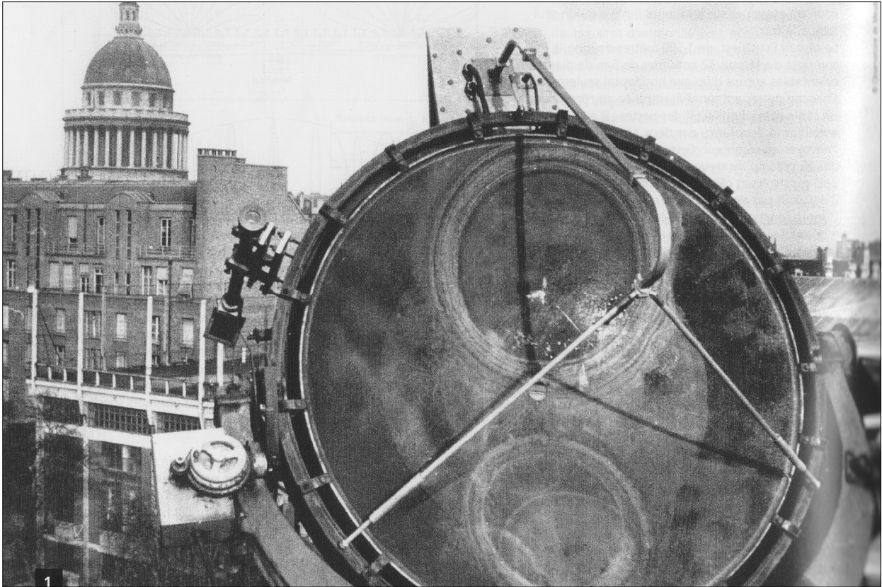
Figure 2: The 1.5m diameter 'searchlight antenna' mounted on the roof of the Physics Laboratory at the ENS in Paris. In the background is the dome of the Panthéon (after Steinberg, 2004: 626).
