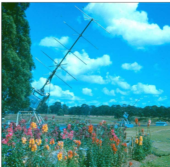
Figure 6: View showing two of the three 97 MHz crossed Yagis comprising Ruby Payne-Scott and Alec Little's solar interferometer. The second Yagi can be discerned behind the colourful garden display maintained by the Water Board (photograph by the author in 1951).
