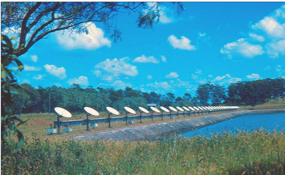
Figure 5: The 32-element solar grating interferometer at Potts Hill photographed on completion in late 1952. The first serious solar observations began in February 1953 (photograph by the author).
