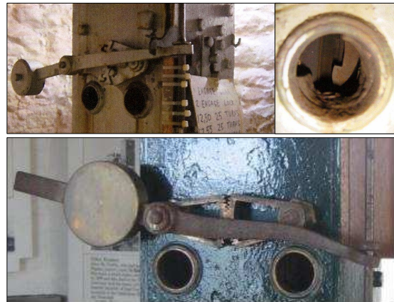
Figure 12: The Edinburgh (top) and Deal (bottom) gear segments and catches (courtesy Allan Marshall and Michael Kinns respectively).
