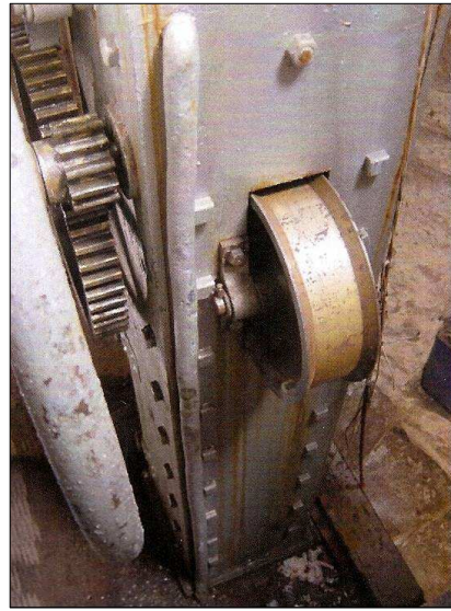
Figure 11: The Edinburgh guide wheel (courtesy: Allan Marshall).
