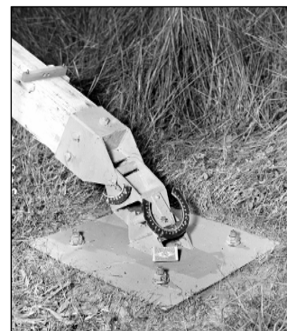
Figure 14: The rhombic aerial's polar mount, with right ascension and declination scales (courtesy: ATNF Historical Photographic Archive).
