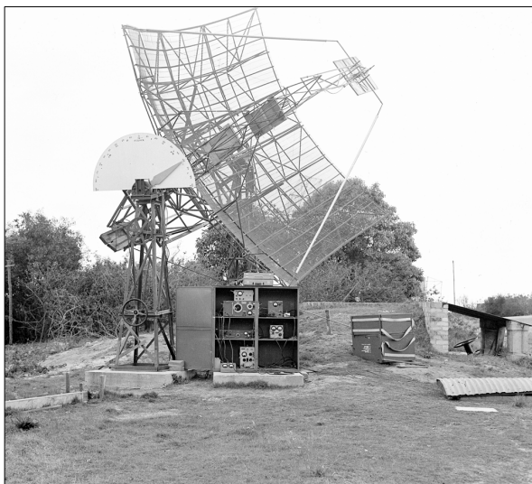
Figure 8: The WWII experimental radar that was used by Lehany and Yabsley at 200, 600 and 1200 MHz to monitor solar emission (courtesy: ATNF Historic Photographic Archive).
