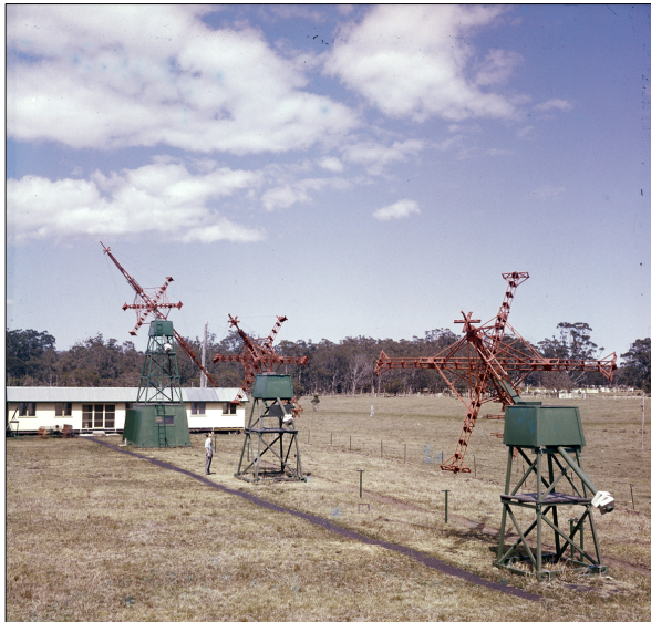
Figure 22: View of the receiver hut and three crossed-rhombic antennas at the Dapto field station (courtesy: ATNF Historic Photographic Archive).
