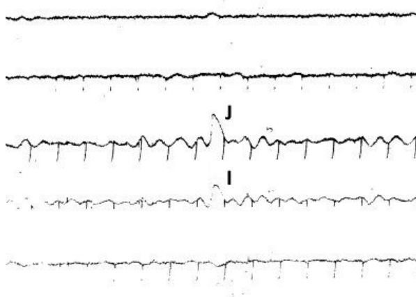
Figure 12: Transit of the radio source Hydra A in a few successive beams of the N-S multichannel array: the source is culminating between lobes I and J (after Joshi, 1962).
