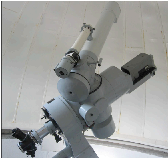
Figure 22: The coudé equatorial of the Ankara Observatory. This instrument has a 15 cm aperture and 2.25 m focal length. It is used for observations of the Sun. The observer stands in a fixed position at the bottom of the polar tube, not as the top as for the Gautier equatorials. The light from the objective is sent to the polar tube by two flat 45° mirrors located on each side of the very short equatorial tube (© Ankara University Observatory).
