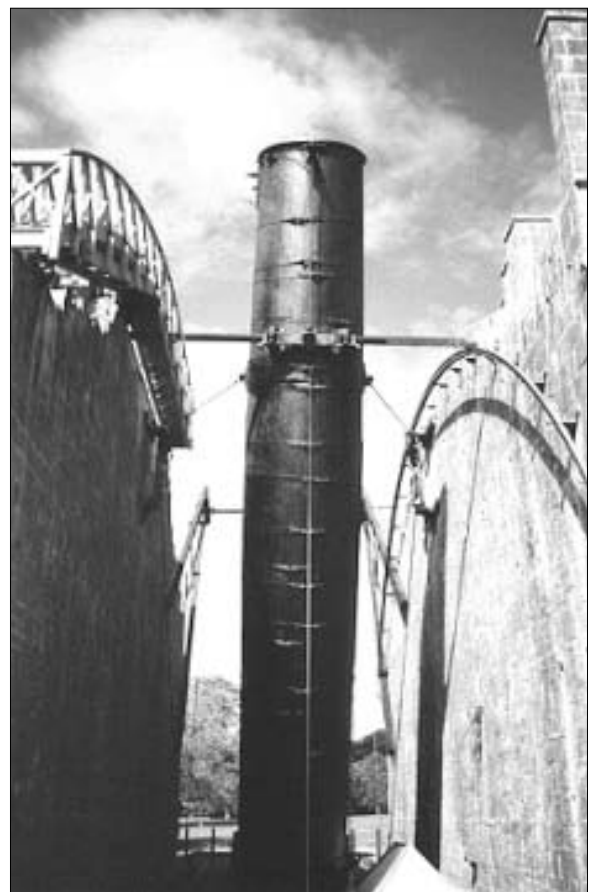
Figure 6: The 72-inch in a near-zenith position. The cross-bar for the azimuthal motion is at the upper third of the 60-foot (18-m) tube; the highest gallery is on top of the western wall (photograph by the author).
