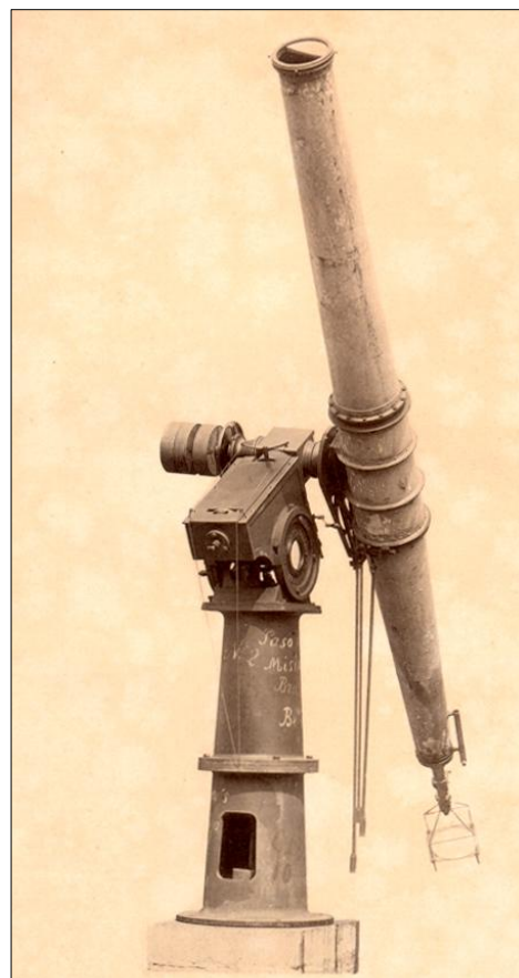
Figure 8: Heliometer with unequal focal lengths (adapted from Sterken et al., 2004: 26).
