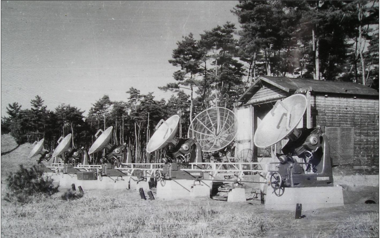
Figure 12: The 5-element E-W grating interferometer in 1953, with the original Toyokawa antenna in the background (courtesy: Tanaka Family).
