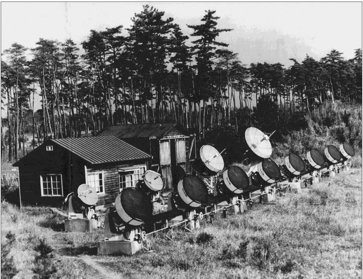
Figure 13: The expanded 8-element solar grating array, complete with polarisation screens, and behind it the four total power radiometers that monitored the Sun at 1000, 2000, 3750 and 9400 MHz (courtesy: Tanaka Family).
