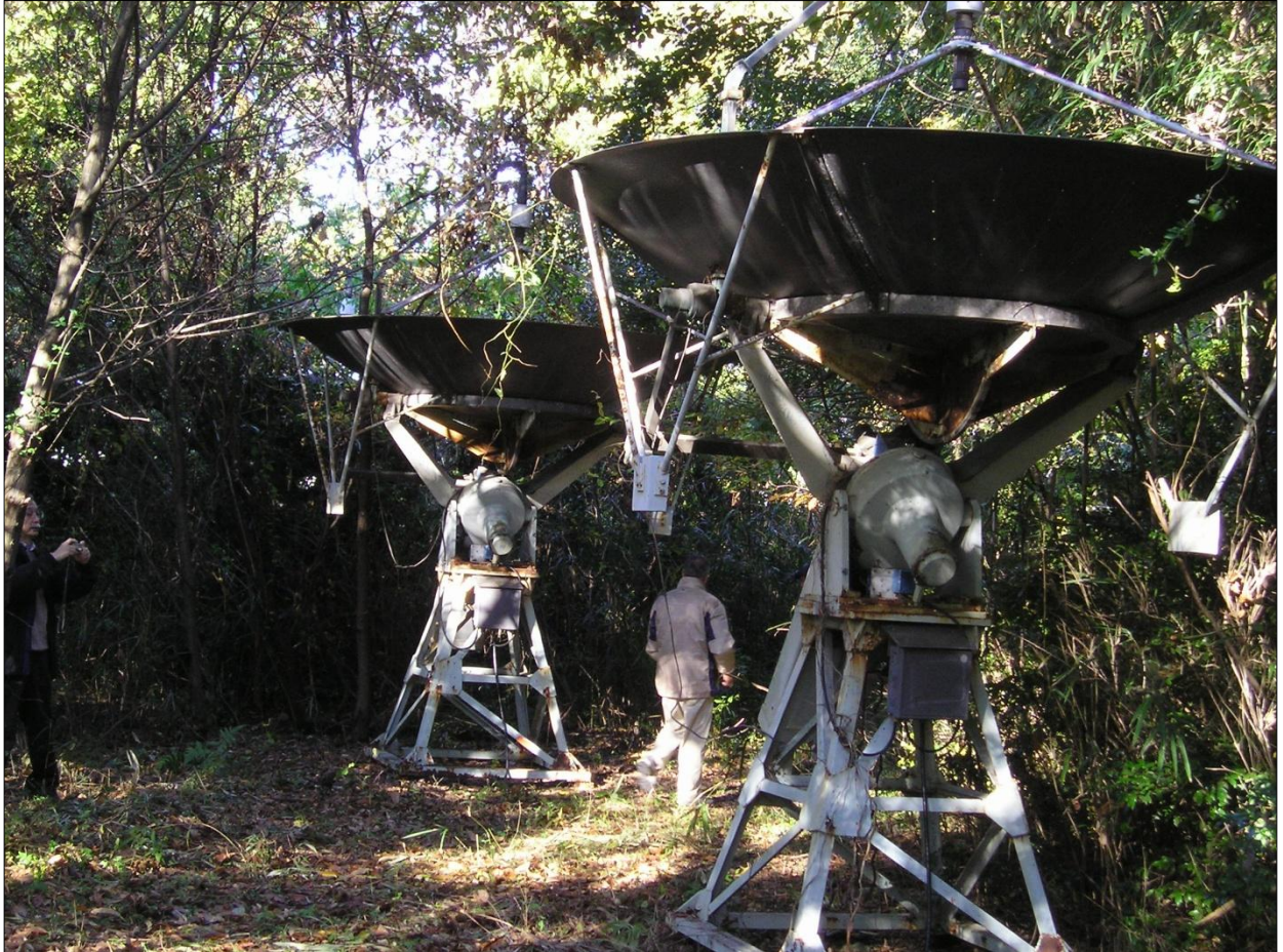
Figure 21: Two of the surviving antennas of a T-shaped array erected in the 1970s, discovered overgrown by dense vegetation just prior to a visit to the Toyokawa Observatory site by the first two authors of this paper in November 2010 (photograph: W. Orchiston).
