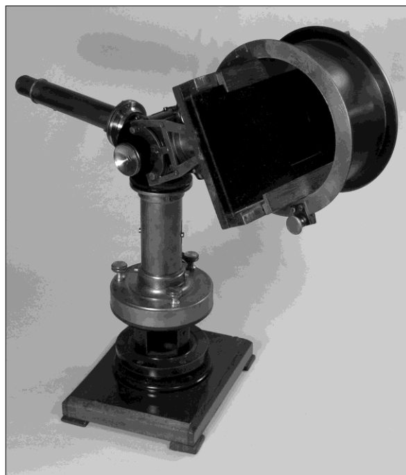
Figure 10: The calcite prism spectrograph (Gothard No 9) made in 1886 (after von Gothard, 1886b).
