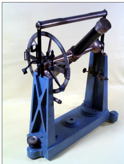
Figure 8: The 27-mm Fraunhofer transit telescope (courtesy: Gothard Astrophysical Observatory Archives).
