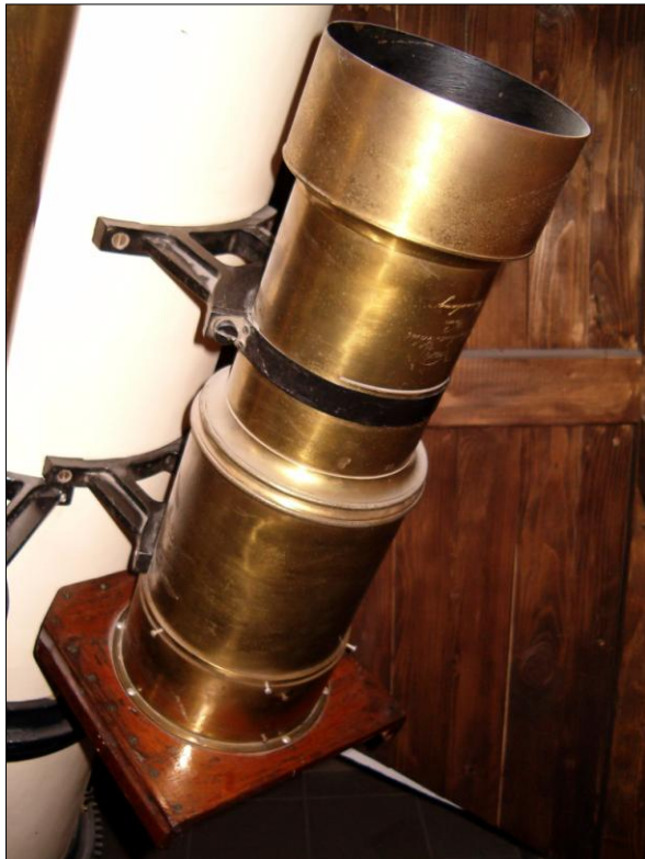
Figure 12: The 10-cm aperture astrograph constructed by von Gothard in 1893 (courtesy: Gothard Astrophysical Observatory Archives).
