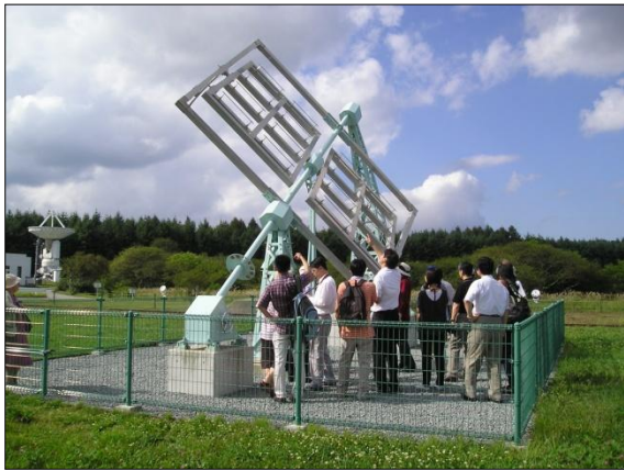
Figure 18: A replica of the original TAO broadside array on display at the Nobeyama Radio Observatory. Only the polar axis is from the original radio telescope of 1949 (photograph: W. Orchiston).
