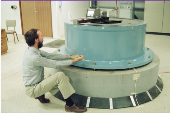
Figure 21: The telescope base being adjusted to accurately level the azimuth bearing mounting face. The measuring apparatus used was that previously devised to measure face flatness during the hand-scraping process.
