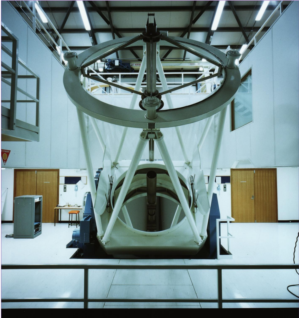
Figure 33: The rotating building places the 2.3m Telescope at the very centre of a laboratory where a variety of instruments can be mounted with ease.
