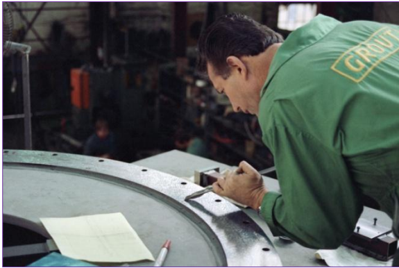
Figure 6: A craftsman in the workshop of John Grout hand-scraping the azimuth-bearing flange of the telescope fork.
