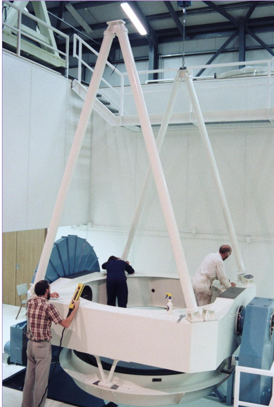
Figure 9: The modified Serurier truss geometry, showing the equal apex angles of the upper and lower trusses.
