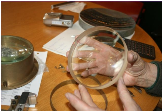
Figure 6: Wolfgang Busch displays the middle (equi-concave) lens element. On the left of the illustration is the brass lens cell. At the top is the mirror, which is thought to have been aluminized in the 1980s for display when the original Schmidt Museum was opened at the Hamburg-Bergedorf Observatory (image courtesy: Walter Stephani and the Hamburg Observatory, University of Hamburg).
