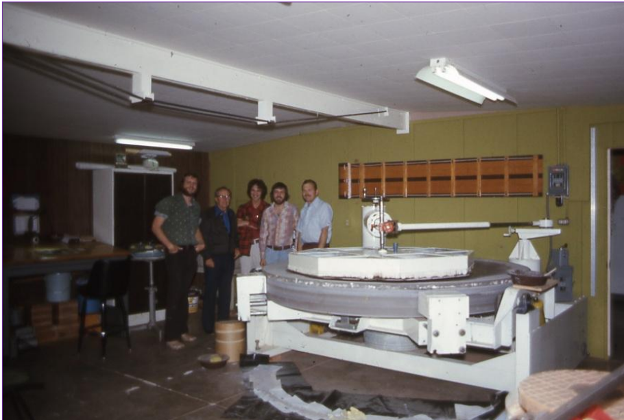
Figure 4: Norman Cole's Optical Shop. Norman is on the right. The blank being machined is that of the 2.3m primary mirror for the Wyoming Telescope (courtesy: R. Gehrz).
