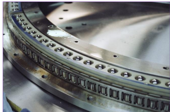
Figure 5: The modified azimuth bearing in the laboratory at Rothe Erde. The upper ring has been removed to show the ball race that provides axial support and the roller race that provides radial constraint.
