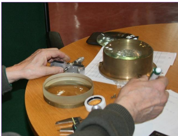
Figure 7: Wolfgang Busch is shown with the spherometer in his left hand which was used to measure the lens radii during the 2007 examination. (image courtesy: Walter Stephani and the Hamburg Observatory, University of Hamburg).
