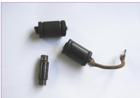
Figure 4: Components of the mixer that Shimoda made in 1948 for the 3,000 MHz receiver.
