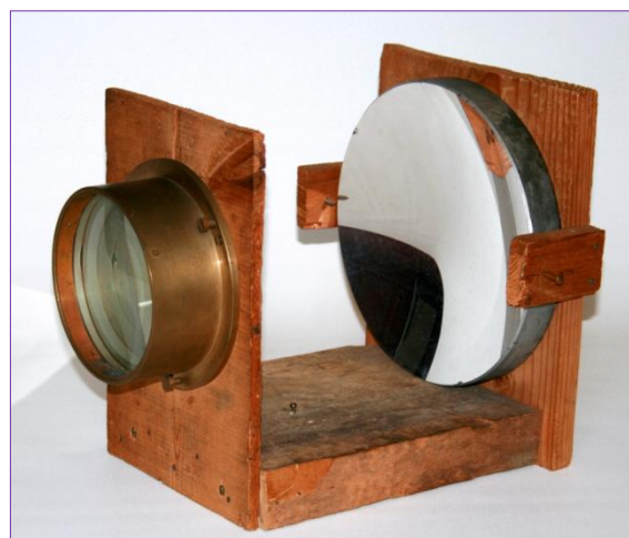
Figure 1: Bernhard Schmidt's prototype camera, consisting of a fast spherical mirror (right), and a 3-lens afocal corrector (left: in a brass lens cell). The optical design is of a type later named 'Buchroeder-Houghton'. Built in 1934, the camera was used by Schmidt to take test images of the sky, shortly before his death (image courtesy: Walter Stephani and the Hamburg Observatory, University of Hamburg).
