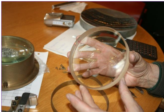
Figure 6: Wolfgang Busch displays the middle (equi-concave) lens element. On the left of the illustration is the brass lens cell. At the top is the mirror, which is thought to have been aluminized in the 1980s for display when the original Schmidt Museum was opened at the Hamburg-Bergedorf Observatory (image courtesy: Walter Stephani and the Hamburg Observatory, University of Hamburg).
