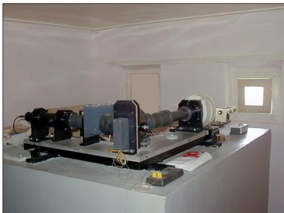
Figure 4: A close-up showing the spectrophotometer at the Kumbel IRIS station (photograph: Sh. Ergamberdiev).
