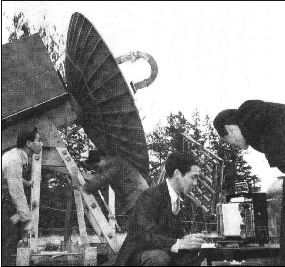
Figure 19: The 3 GHz parabolic antenna which was used to observe the partial solar eclipse in Tokyo on 14 February 1953 (courtesy: K. Akabane).
