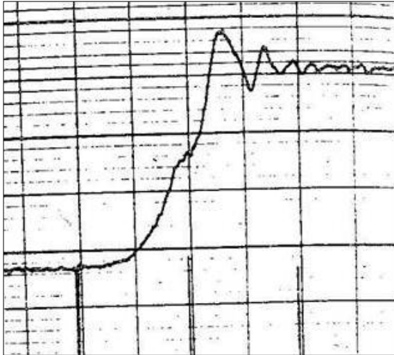
Figure 9: Chart record showing the immersion of the radio source 3C 273 behind the Moon on 5 August 1962 at 410 MHz. Time runs from right to left. The right hand (early) part of the curve shows the Fresnel diffraction pattern as the smaller component B is occulted, followed by the disappearance of the larger component, A (after Hazard et al., 1963; reproduced with permission).
