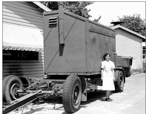
Figure 13: The ex-Army radar trailer in the grounds of the Radiophysics Laboratory. This mobile radio telescope featured four Yagi aerials, a new 100 MHz receiver, recorders, chronometers, weather recording instruments and all the tools and backup equipment needed to operate reliably at a remote location. We were not able to establish the identity of the lady in the photograph (courtesy: RAIA B1259).
