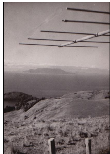
Figure 15: The mobile radio telescope on the Greenwood farm at Pakiri Hill in June 1948. The cabin mounted on the trailer could swivel in azimuth to observe sources rising at different declinations along the horizon (courtesy: Stanley family).
