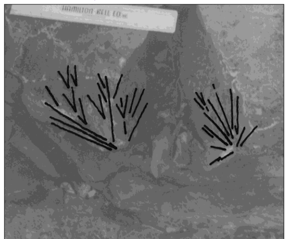
Figure 19: Use of an overlay to indicate the features that may be shatter cones (after Woodruff, 1968: 24).
