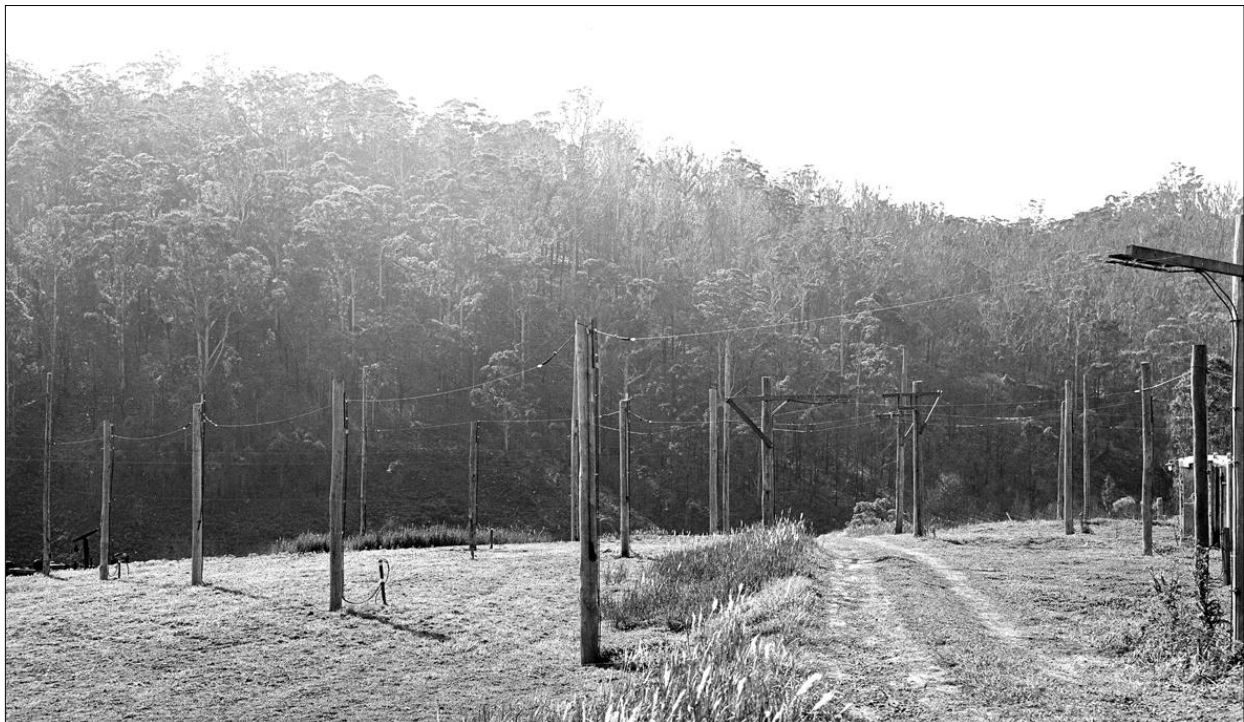
Figure 16: A photograph showing part of the second 18.3 MHz array at Hornsby Valley. Once again, the ground served as a reflector (courtesy: CSIRO RAIA B2802-5).
