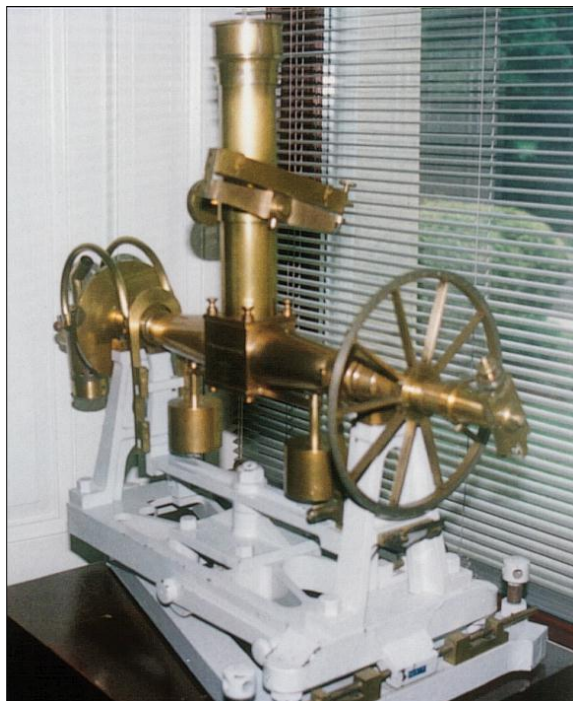
Figure 4: One of the Stackpole broken tube transit telescopes used to observe the 1874 transit of Venus, and now at the U.S. Naval Observatory (photograph: Wayne Orchiston).
