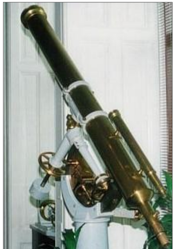
Figure 5: One of the 5-in Alvan Clark refractors used to observe the 1874 transit of Venus, and now at the U.S. Naval Observatory (photograph: Wayne Orchiston).
