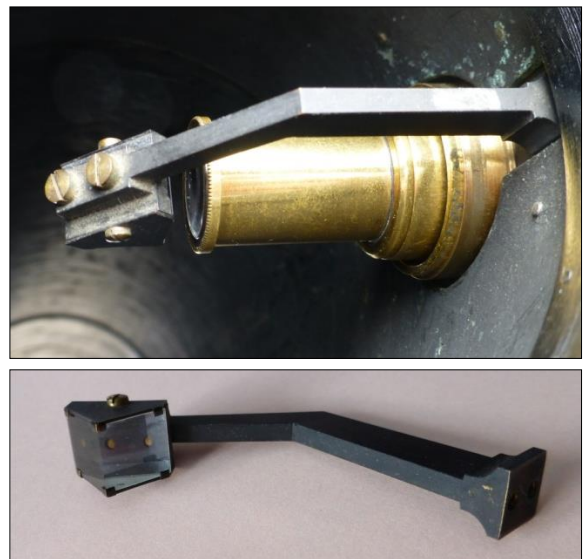
Figure 57: Secretan No. 13 10-cm reflector, prism assembly (upper) in position, and (lower) removed (author's photographs).
