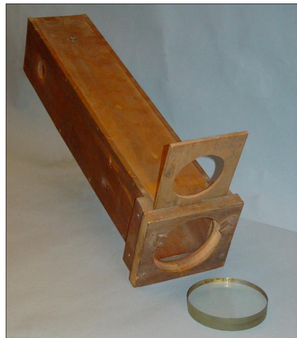
Figure 4: Probably Foucault's first telescope from January 1857 (Paris Observatory inv. 251). The aperture stop that slots at the front of the mirror cell has been raised to be more evident. Its diameter is 3\frac{1}{4} French inches ( pouces ) or 88 mm. The focal length of the mirror is 530 mm, corresponding to an f/6.0 focal ratio (courtesy: Observatoire de Paris/F. Auffret).
