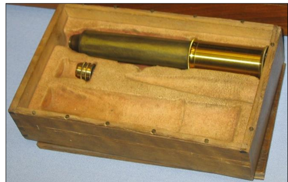
Figure 20: (Upper) Eyepiece box of the Prytanée No. 2 telescope, with the 'blunt' style of eyepiece assembly (courtesy: L. Chanteloup/PNM). (Lower) Eyepiece box of the Science Museum No. 26 telescope with an eyepiece assembly like the 'simplified achromatic microscope' seen in Figure 19. Three nosepiece lenses have been unscrewed from the associated tube. An indentation for the blunt assembly is seen; the blunt assembly itself is pictured at collectionsonline.nmsi.ac.uk (author's photograph). A note attached to the No. 2 box indicates that the cone-like indentation was provided for a dust brush. Another indentation present in both boxes must be for the eyepiece of the finder that equips each instrument (see text).
