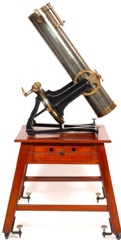
Figure 67: Metal-mounted 16-cm Foucault-Secretan telescope No. 18, dated 1866. In 1880 it was purchased by José Batlle y Ordóñez (1856–1929), who was later President of Uruguay. The polar axis is set for a latitude of 35°, which is correct for Montevideo, but the hour-angle circle is labelled for the northern hemisphere (courtesy: E. Wolf).
