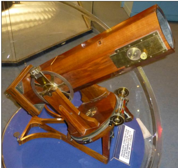
Figure 38: Palais de la Découverte telescope, formerly the property of Félix Worms de Romilly. The sliding focusing plate and control knob are visible at the front of the tube (cf. Figures 7 and 40) but the eyepiece has been removed and its mounting hole covered with a circular brass plate (see text). The highly-polished octagonal tube is decorated with a slight step close to the position of the declination axis. The handle of one of two hand cranks for tracking in hour angle can be seen (author's photograph).
