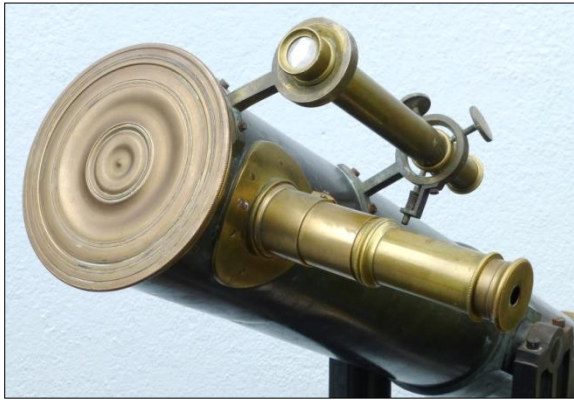
Figure 54: Secretan No. 13 10-cm reflector, view of eyepiece, brass dust cap, finder and finder-alignment mechanism. The weighty dust cap with bayonet pins and crudely-cut slots to retain it (not visible) looks to be a replacement. Any lost cap must have been held on by friction, because there is no screw thread on the tube, unlike other 10-cm instruments (author's photograph).
