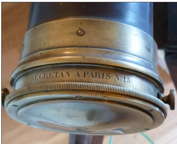
Figure 55: Secretan No. 13 reflector, mirror cell, maker's mark and serial number (author's photograph).
