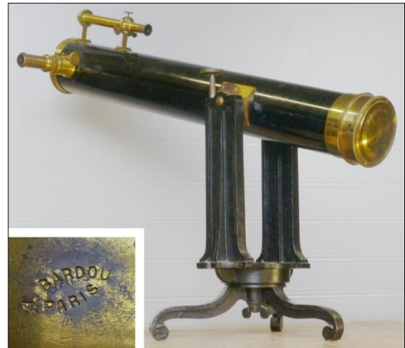
Figure 94: 4-pouce telescope belonging to the Lycée Janson de Sailly in Paris. The inset shows A. Bardou’s name stamped at centre rear of the mirror cell (author’s photographs).
