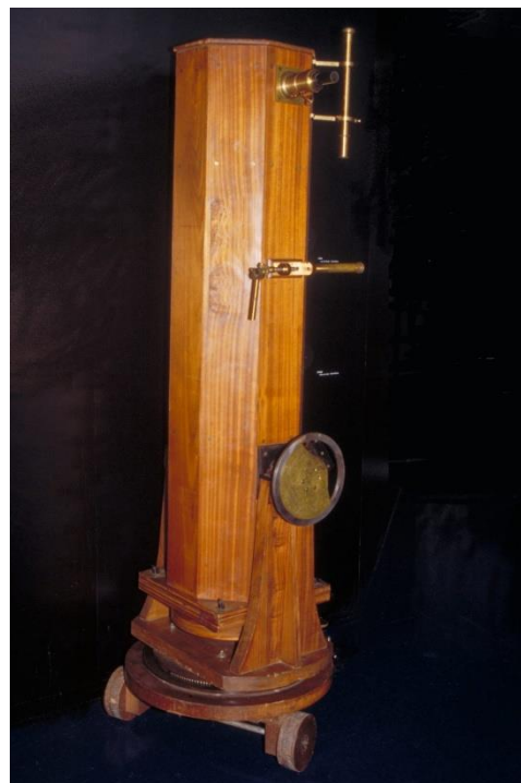
Figure 97: Wooden-tubed telescope attributed to “Ateliers R. Mailhat 1857–1868”. The dates are improbable, because though similar to Foucault-Secretan wooden tubes, there are differences of detail (such as the round wooden mirror cell and the form of the fork) and the Mailhat firm dates from 1894 (after: Musée des Confluences, 2009: 50).
