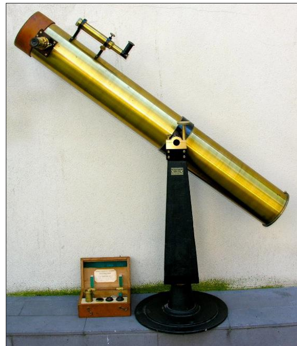
Figure 85: A surviving example of the simplified telescope. The cap is leather (courtesy: www.astrobin.com).
