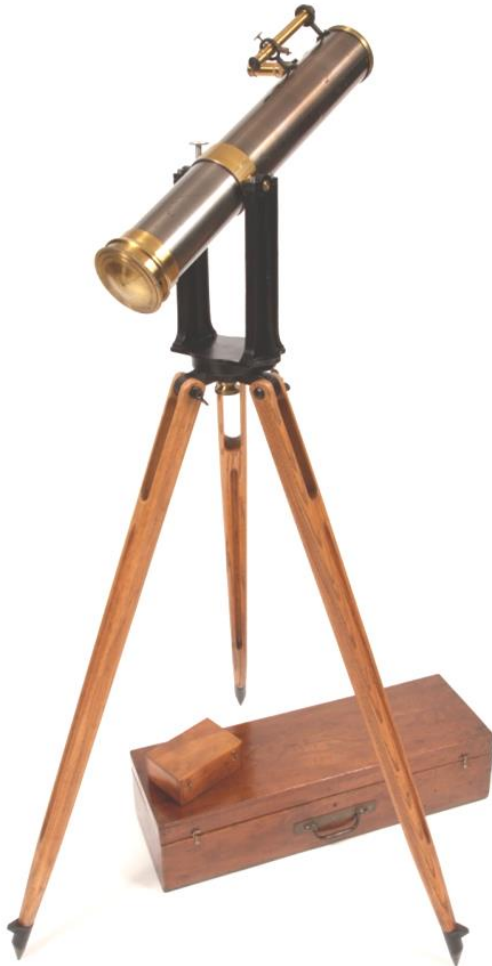
Figure 62: General view of 10-cm telescope from the Wolf collection, Secretan serial No. 236, dated to 1888–1894. The tripod is similar to that equipping telescope No. 13, but the eyepiece barrel diameter is less (see Table 11) (courtesy: E. Wolf).
