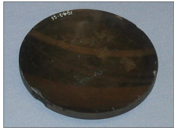
Figure 3: Tarnished silvered mirror roughly 100 mm in diameter given to Sir John Herschel when Foucault visited him at Collingwood on 11 September 1857. The mirror is much faster than those made by Foucault for astronomical use, who also gave Herschel a sector of platinized glass. The interest appears to have been methods for making glass reflective. The two items are now in the Science Museum, London, inventory 1943-55 (author's photograph).
