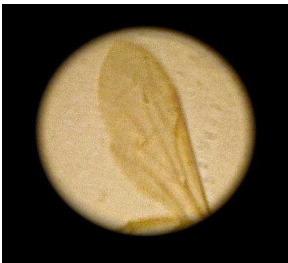
Figure 22: The Wolf 4- pouce telescope used to image a wasp's wing. A ~2-cm aperture was used to select the best part of the surviving mirror silvering. It was possible to focus on the specimen placed about 4 m in front of the mirror with the eyepiece assembly still just held by the rack-and-pinion mounting sleeve. Field diameter ~8.4 mm (courtesy: Ed Wolf).
