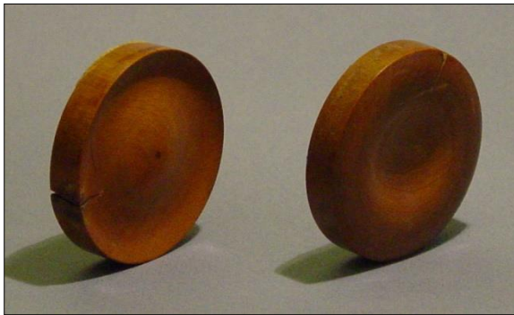
Figure 24: Wooden models used by Foucault when explaining his knife-edge test (Paris Observatory, inv. 244). The test reveals errors of form in exaggerated relief. At left, there has been too much polishing in a ring midway between centre and edge. At right, the center is overpolished and the edge is turned down (courtesy: Observatoire de Paris/F. Auffret).
