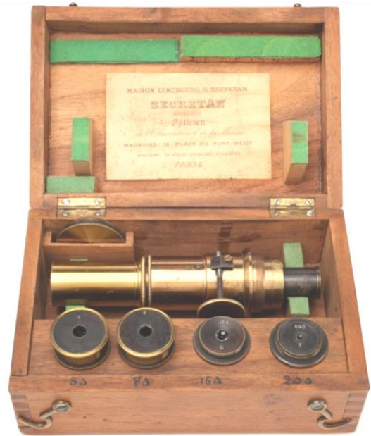
Figure 64: The eyepiece box for telescope No. 236. When the eyepiece assembly is removed from the telescope tube, dust can be prevented from entering with the cap seen at upper left. The misprint "Maison Lerebourg & Secretan" on the business card surprises, but less-so when it is understood that in French "Lerebourg" and "Lerebours" are homophonous. The card gives 30, rue du Faubourg Saint-Jacques as the workshop address (cf. Table 1 and Section 9.2) (courtesy: E. Wolf).
