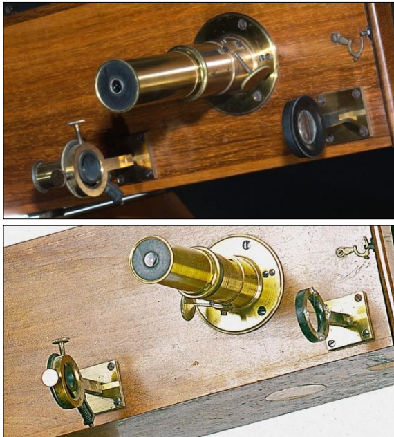
Figure 21: Comparison of the finder provisions on the two Prytanée télescopes . No. 2 (upper) is provided with an eyepiece and objective lens (see also Figure 17). Thumb-screws and a sprung-loaded pin permit optical alignment with the main telescope. For No. 3 (lower) the arrangement is purely geometric. A peep-hole defines a viewpoint for a sighting ring. Cross hairs have subsequently been soldered across this ring, but are unlikely to have been effective owing to the eye's inability to focus simultaneously on a nearby object and the sky (courtesy: L. Chanteloup/PNM).
