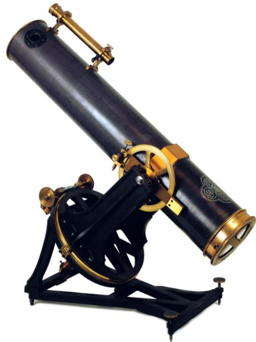
Figure 70: A similar 16-cm telescope to that shown in Figure 67, described by Bennett (2009: 566) as one of the "... highlights ..." of the Musée Gassendi in Digne. The eyepiece assembly is missing. The curved mirror rear rests against a matching curved metal cross, which arrangement probably facilitates collimation. The instrument was restored in 1991 (Turner, 2006). The arms of the original owner are engraved on the tube (courtesy: Collection Musée Gassendi, Digne-les-Bains).
