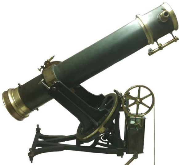
Figure 78: 16-cm telescope with motor drive offered for sale by Christie's South Kensington in 2008 (see Table 9). The original mirror and cell are missing and have been replaced, so there is no signature or serial number. The eyepiece lenses are also lost. Like the Milan telescope (Figure 93), the tube has an additional external ring (courtesy: J. Duncan).
