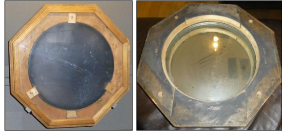
Figure 36: Front (left) and rear views of a 330-mm mirror attributed to Foucault conserved by the Musée des Arts et Métiers in Paris. The focal length claimed on a paper label is 2.29 m, close to the 2.25 m announced by Foucault. One might think that the octagonal wooden cell once formed part of a telescope. In this case, the black marks visible in the rear view would be paint to reduce reflections and the mirror would now be reversed for display purposes. But if this were the case, one would also expect the exposed circular cut of the wood around the mirror to be blackened too. The mirror is made of clear glass. The tarnished concave surface is protected behind an octagonal sheet of thin glass (author's photographs).
