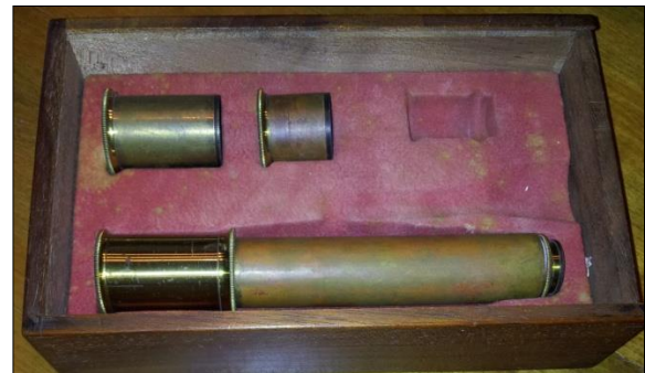
Figure 19: Lerebours' simplified achromatic microscope sold with three stackable nosepiece lenses, rack-and-pinion focusing and even a right-angle prism option (not illustrated) for horizontal use. The similarity with certain of the Foucault-Secretan telescopes is evident (after: Lerebours and Secretan, 1853: 7; courtesy: Universiteitsbibliotheek Gent via Google Books).
