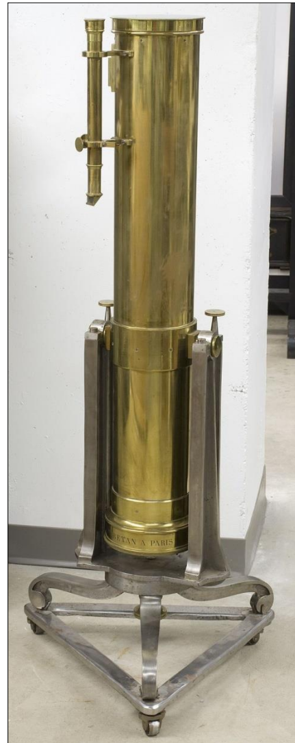
Figure 76: Alt-azimuth 16-cm reflecting telescope conserved at Harvard University (see Table 9). Two locking screws are provided for the altitude axis (cf. Figure 53). The eyepiece assembly is not attached, but is similar to those of other metal-mounted instruments (courtesy: Collection of Historical Scientific Instruments, Harvard University).
