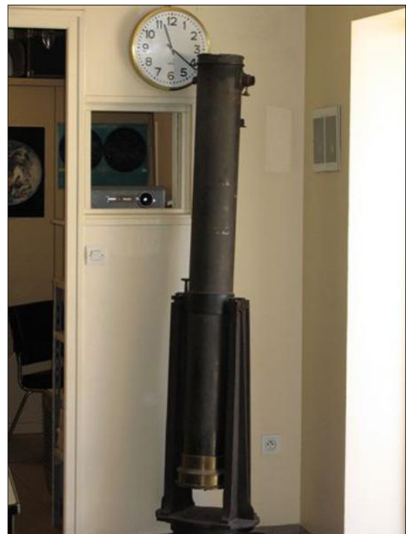
Figure 80: Secretan 16-cm alt-azimuth reflector at the Observatoire de Rouen dating from 1884 (see Table 9). The focal ratio is \sim f/10 (courtesy: www.astrosurf.com/obsrouen ).
