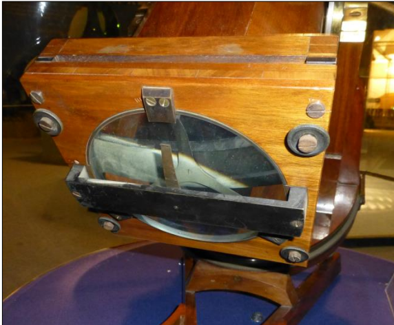
Figure 42: The rear of the Palais de la Découverte mirror and mirror cell. The mirror rear was polished to permit monitoring of the silver deposition on the front (Foucault, 1859a). Heads are visible for four pairs of counteracting screws that provide for alignment of the optical axis of the mirror (author's photograph).
