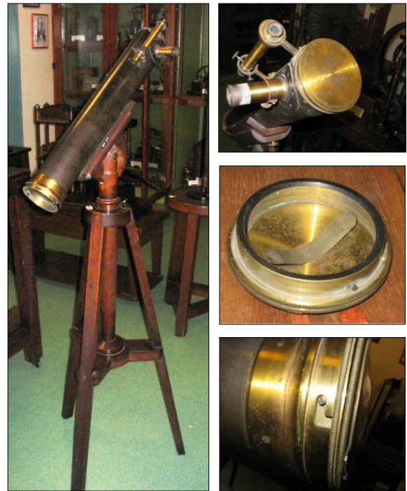
Figure 52: 10-cm telescope at the Lycée Louis le Grand in Paris. There is no signature or serial number. Clockwise from left: (a) Overall view. Is the tripod original or a substitution? It is more stable than the one equipping Nos 13 or 236 (Figures 53 and 62), the legs of which easily splay open. (b) View of the front of telescope and dust cap, which screws on. (c) Mirror cell and spring. The mirror has been lost. (d) Bayonet attachment of the mirror cell to the telescope tube (author's photographs).
