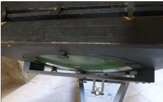
Figure 28: To improve strength while minimizing weight, the mirror of the Paris Observatory 40-cm reflector has a curved back, which was polished for monitoring progress during silvering. The mirror is no longer held on an air bag. The green tint is characteristic of St Gobain crown glass (author’s photograph).
