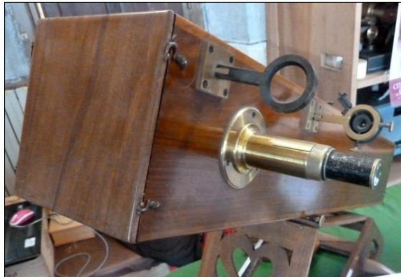
Figure 16: No. 42 9-cm telescope, with eyepiece assembly held by friction, geometric finder and what appears, from the match of the wood, to be an original square dust shutter. The serial number is marked on the body of the instrument and is also engraved on the glass in writing that resembles Foucault's writing (Fuentes, pers. comm., 2015) (after: www.astrosurf.com/rtaa/rtaa2011_expo.html ).
