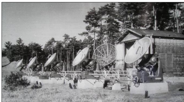
Figure 9: A view of the 4 GHz five-element grating interferometer installed at Toyokawa in 1953 (courtesy: Tanaka Family).
