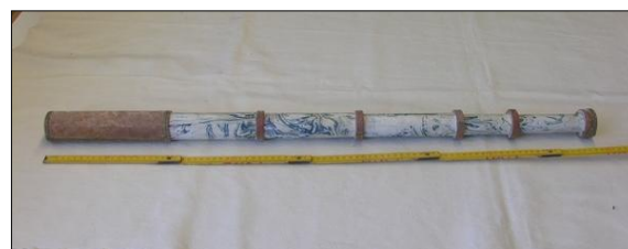
Figure 13: The world’s oldest-known surviving telescope, which is securely dated to 1617, is now in the Kunstgewerbemuseum/Staatliche Museen zu Berlin. The maker is unknown. This cloth and paper telescope comprises a main tube, and five draws of pasteboard. Each draw is covered in marbled paper. The end tube and ring stops are in silk velvet embroidered by gold thread. When collapsed the end tube and rings have a common outer diameter of 48mm (after http://dioptrice.com/telescopes/782 ).
