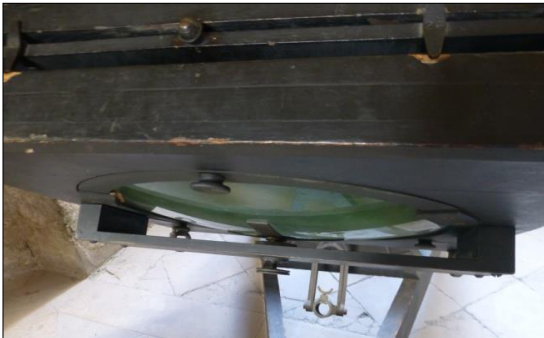
Figure 28: To improve strength while minimizing weight, the mirror of the Paris Observatory 40-cm reflector has a curved back, which was polished for monitoring progress during silvering. The mirror is no longer held on an air bag. The green tint is characteristic of St Gobain crown glass (author's photograph).
