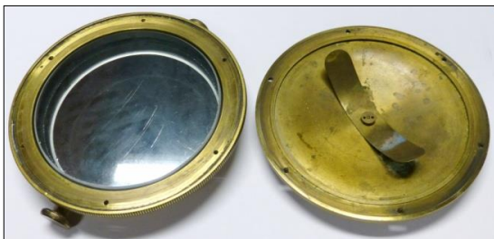
Figure 56: Secretan No. 13 reflector, mirror-cell back removed showing the clear glass and flat rear of the 100-mm mirror and the leaf spring that keeps it in position (author's photograph).
