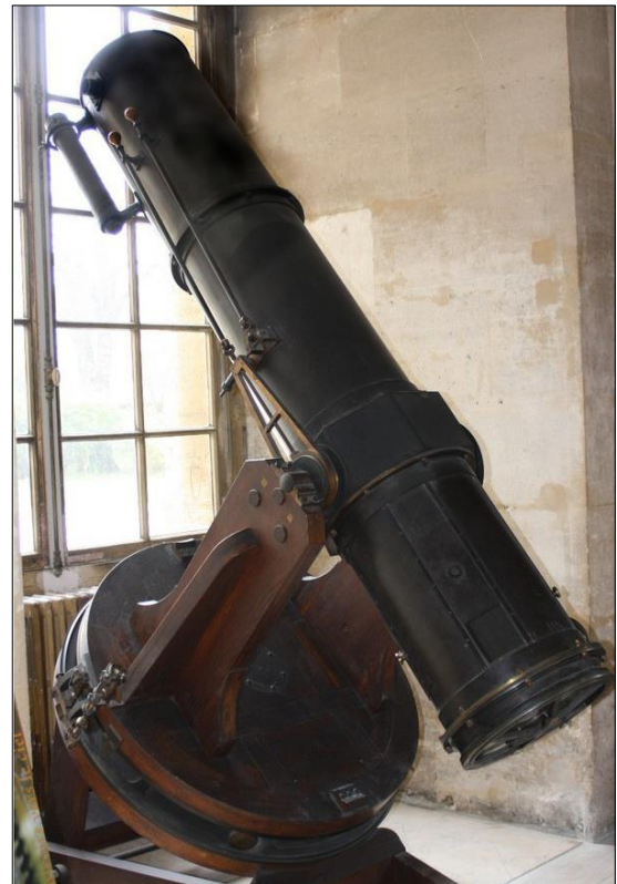
Figure 73: Not a Foucault-Secretan telescope! This 40-cm reflector for the Paris Observatory was completed in 1871. The mirror was figured by Martin for a cost of 2,400 fr (Martin, 1870c). The mechanical work, the 25-mm crown-glass prism and achromatic eyepiece were supplied by Eichens (6,500 fr: Eichens, 1871b). The tube is metallic. Although metal tubes reduce chimney currents, it was found necessary to insert four aeration vents near the mirror some months later (Eichens, 1872). The lower control rod locks the triangular structure in declination. The upper rod serves to move the tube against the structure, so providing fine control. The declination circle on the other side of the tube is very similar to the one on the Foucault-Secretan 40-cm telescope (Figure 27) (courtesy: astro2009.futura-sciences.com and X. Plouchart).
