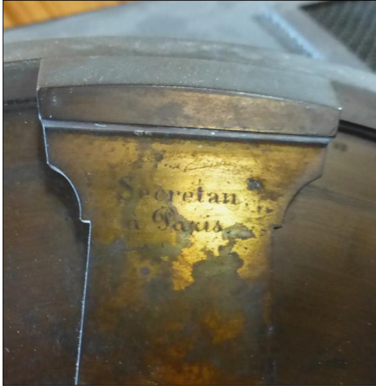
Figure 27: The 40-cm telescope is signed "Secretan à Paris" near the declination circle. The cursive font is also found in the firm's signature on photographic lenses. There is no lock or fine adjustment (cf. Figure 41), these functions being provided by the rod and hinged plank seen in Figure 26 (author's photograph).
