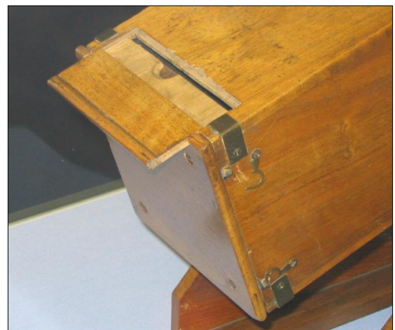
Figure 15: Access hatch to the mirror dust slide of the Science Museum telescope No. 26 (author's photograph).
