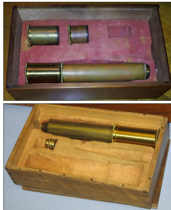
Figure 20: (Upper) Eyepiece box of the Prytanée No. 2 telescope, with the 'blunt' style of eyepiece assembly (courtesy: L. Chanteloup/PNM). (Lower) Eyepiece box of the Science Museum No. 26 telescope with an eyepiece assembly like the 'simplified achromatic microscope' seen in Figure 19. Three nosepiece lenses have been unscrewed from the associated tube. An indentation for the blunt assembly is seen; the blunt assembly itself is pictured at collectionsonline.nmsi.ac.uk (author's photograph). A note attached to the No. 2 box indicates that the cone-like indentation was provided for a dust brush. Another indentation present in both boxes must be for the eyepiece of the finder that equips each instrument (see text).
