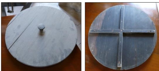
Figure 29: The dusty tube cap for the 40-cm reflector is made of thin wood strengthened with a wooden cross which also acts to hold the cap in position in the tube (author's photographs).
