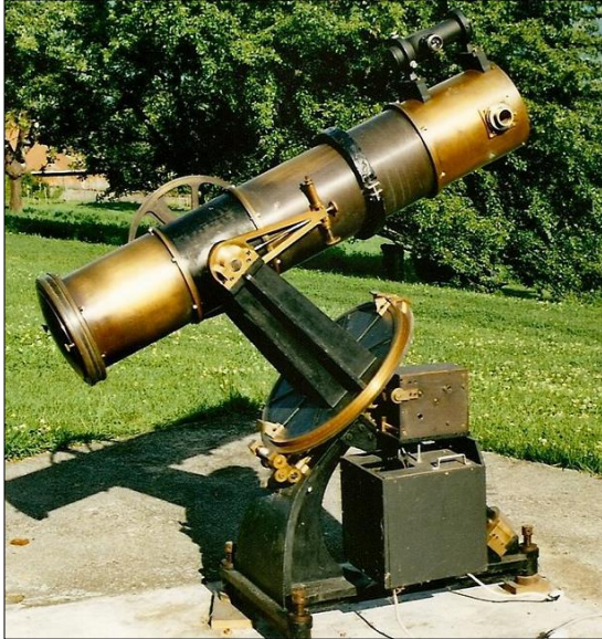
Figure 81: An equatorial 200-mm Foucault-Secretan telescope dated 1877 belonging to the Groupe d'Astronomie du Dauphiné (GAD) (see Table 9). The GAD received it as a gift from the University of Grenoble and electrified the drive (Pouget, pers. comm., 2015). The finder telescope differs from those shown in Figures 82 and 83, suggesting it is a replacement (courtesy: G. Auzet).
