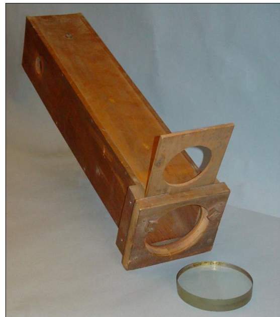
Figure 4: Probably Foucault's first telescope from January 1857 (Paris Observatory inv. 251). The aperture stop that slots at the front of the mirror cell has been raised to be more evident. Its diameter is 3\frac{1}{4} French inches ( pouces ) or 88 mm. The focal length of the mirror is 530 mm, corresponding to an f/6.0 focal ratio (courtesy: Observatoire de Paris/F. Auffret).
