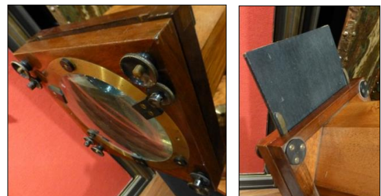
Figure 100: The telescope auctioned at the Hôtel Drouot in November 2015. For an assessment, see Section 12.2. (Top) Overall view. The base measures 360 × 362 mm. Unlike the de Romilly telescope (Figure 38), the slats composing the octagonal tube have no decorative step. Their exposed length is 930 mm. Now in the collection of Vivek Hira, New York (courtesy: galerie-liova.com). (Bottom left) Mirror cell and (bottom right) mirror dust slide (author's photographs).
