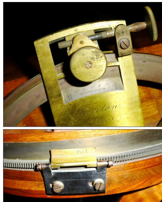
Figure 41: (Upper) Details of the declination setting circle, vernier and Secretan's name for the Palais de la Découverte telescope. The circle is calibrated in terms of north polar distance, 180°–0°–180°. The face-on knurled knob is the declination lock; the side-on screw is a fine adjustment. (Lower) Hour-angle circle, numbered 1–24 in hours increasing westwards, in accordance with the normal convention of a target's hour angle increasing with time (author's photographs).
