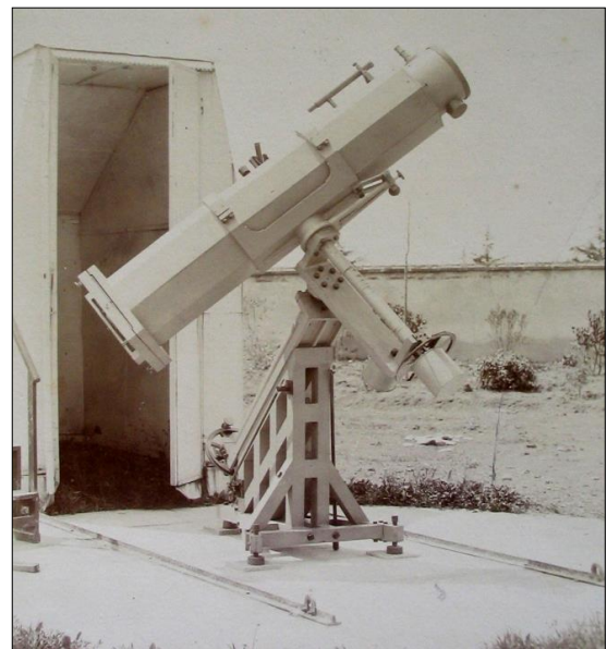
Figure 35: Toulouse Observatory's 33-cm Foucault telescope, much modified. Initially mounted as an alt-azimuth, an equatorial mount was under construction in 1863 (Petit, 1863). The base was strengthened in 1874 by Brunner. This photograph dates from after 1891, the year when a cast-iron mount by Eichens was installed, salvaged from another telescope (Lœwy, 1891), but before the tube was replaced with a metal one (Baillaud, 1899) (author's photograph from an original at the Paris Observatory).
