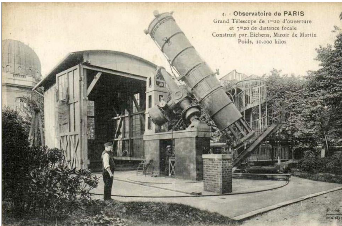
Figure 75: The 120-cm reflecting telescope, enclosure and helical observing platform. Proposed in 1862, the mirror blank was cast the following year, but the telescope was not completed until 1876. The optics never performed satisfactorily. Paris Observatory’s east wing and dome are visible in the background (courtesy: www.cparama.com ).
