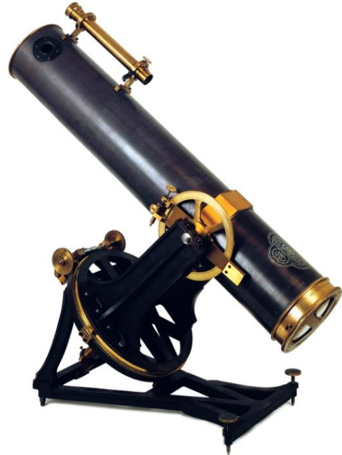
Figure 70: A similar 16-cm telescope to that shown in Figure 67, described by Bennett (2009: 566) as one of the "... highlights ..." of the Musée Gassendi in Digne. The eyepiece assembly is missing. The curved mirror rear rests against a matching curved metal cross, which arrangement probably facilitates collimation. The instrument was restored in 1991 (Turner, 2006). The arms of the original owner are engraved on the tube (courtesy: Collection Musée Gassendi, Dignes-Bains).
