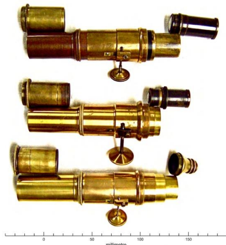
Figure 69: Eyepiece assembly comparison for the three Wolf collection telescopes with eyepiece and relays lenses detached. (Upper) 16-cm telescope, No. 18. (Middle) 10-cm telescope, No. 236. (Bottom) 4-pouce telescope, No. 4. In all cases, friction holds the 'microscope' barrel in the rack-and-pinion focus slider, which has a throw of about 2½ cm (courtesy: E. Wolf).
