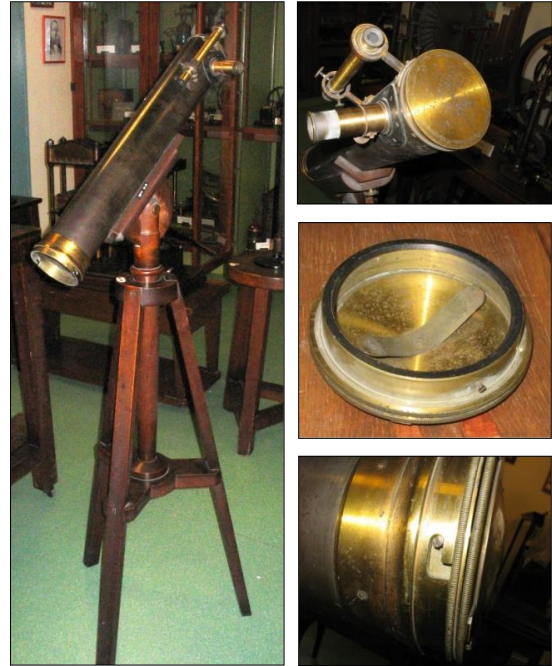
Figure 52: 10-cm telescope at the Lycée Louis le Grand in Paris. There is no signature or serial number. Clockwise from left: (a) Overall view. Is the tripod original or a substitution? It is more stable than the one equipping Nos 13 or 236 (Figures 53 and 62), the legs of which easily splay out. (b) View of the front of telescope and dust cap, which screws on. (c) Mirror cell and spring. The mirror has been lost. (d) Bayonet attachment of the mirror cell to the telescope tube (author's photographs).
