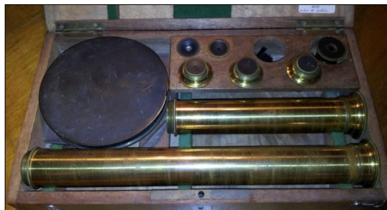
Figure 60: Accessories box for the No. 61 telescope. At upper left is the covered mirror sub-cell. The long tubes are terrestrial eyepieces while the small eyepieces are for celestial use (courtesy: L. Chanteloup/MNP).
