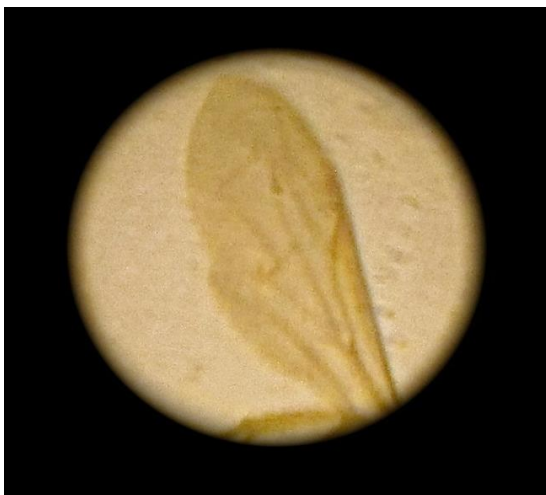
Figure 22: The Wolf 4-pouce telescope used to image a wasp's wing. A ~2-cm aperture was used to select the best part of the surviving mirror silvering. It was possible to focus on the specimen placed about 4 m in front of the mirror with the eyepiece assembly still held by the rack-and-pinion mounting sleeve. Field diameter ~8.4 mm (courtesy: Ed Wolf).
