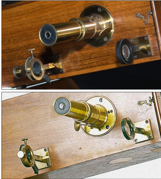
Figure 21: Comparison of the finder provisions on the two Prytanée telescopes. No. 2 (upper) is provided with an eyepiece and objective lens (see also Figure 17). Thumb-screws and a sprung-loaded pin permit optical alignment with the main telescope. For No. 3 (lower) the arrangement is purely geometric. A peep-hole defines a viewpoint for a sighting ring. Cross hairs have subsequently been soldered across this ring, but are unlikely to have been effective owing to the eye's inability to focus simultaneously on a nearby object and the sky (courtesy: L. Chanteloup/PNM).
