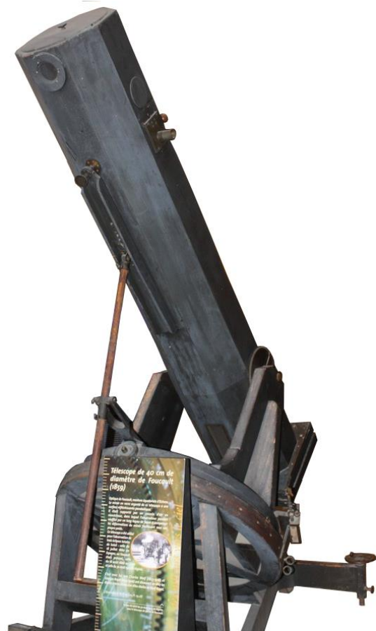
Figure 26: The 40-cm telescope made by Foucault and Secretan for the Paris Observatory in 1859 (inv. 212). The original eyepiece assembly has been replaced. Coarse adjustment in declination is achieved via the support rod. Fine adjustment is provided by a screw engaging the underneath of the tube (cf. Figure 31) (courtesy: astro2009.futura-sciences.com and X. Plouchart).
