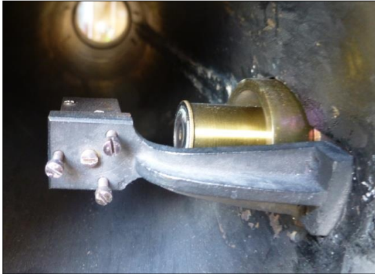
Figure 95: Prism arm of the Janson de Sailly 4-pouce telescope. The arm in the Milan telescope (Figure 93) is similar, and provides a distinguishing feature from Secretan instruments (e.g. Figures 17, 46 and 57) (author's photograph).
