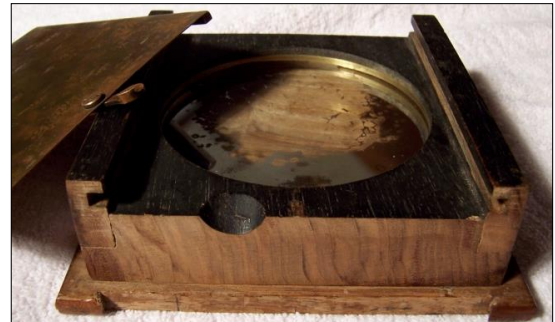
Figure 14: Mirror cell of the Wolf telescope No.4 before renovation. The copper dust slide is disengaged. The silvering is absent in places and heavily tarnished elsewhere (courtesy: Ed Wolf).
