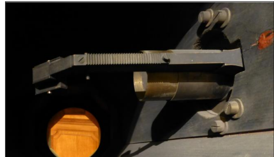
Figure 46: (Upper) The Paris Observatory 20-cm telescope is characterized by the 200-mm diameter aperture at the front of the tube. (Lower) A rack gear attached to the arm supporting the prism is no doubt part of the device used to support and adjust the photographic plate in Wolf and Rayet's lunar-eclipse photography in 1865. The opposite edge of the arm shows wear marks, as from a moveable carriage (author's photographs).
