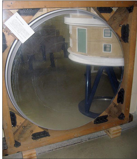
Figure 87: Martin's mirror from the Paris 120-cm telescope was refigured in the 1930s by the optician André Couder and installed in 1942 at the Observatoire de Haute-Provence. The mirror was chipped soon afterwards and is now on display at the Observatory. The damage has been hidden by the large bevel (courtesy: www.obs-hp.fr ).
