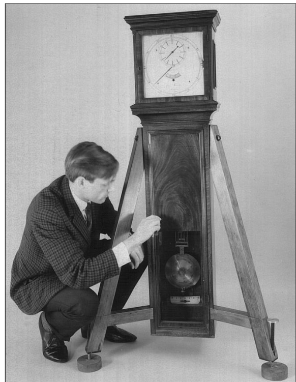
Figure 32: Shelton astronomical clock RS35, showing the replica tripod support (courtesy: the late Derek Howse).
