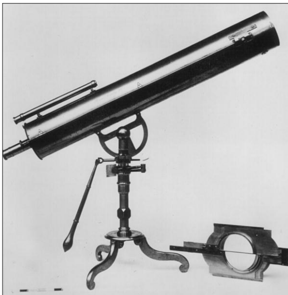
Figure 12: A Gregorian telescope by James Short, very similar if not identical to the ones that accompanied Cook and Green to Tahiti. At the bottom right is an object-glass micrometer that was used for measuring the angular separation of Venus from the limb of the Sun in the course of the transit (courtesy: The Royal Society, London).
