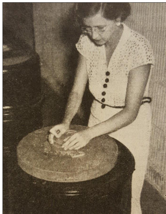
Figure 1: Mirror grinding (after Barton and Joseph, 1951: 171).
