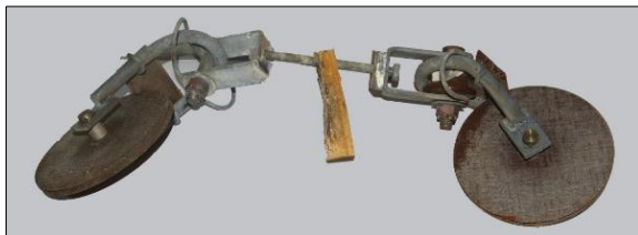
Figure 9: A pair of pulleys that were mounted atop a tall pole. The east and west components of each dipole passed over the pulleys then dropped down to a few metres above the ground (photograph: Martin George; courtesy Estate of Grote Reber).
