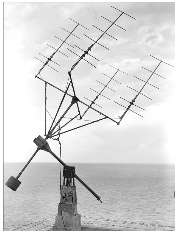
Figure 7: The 200 MHz 4-element Yagi array on the roof of the blockhouse at Dover Heights (courtesy: CRAIA B1165-2).
