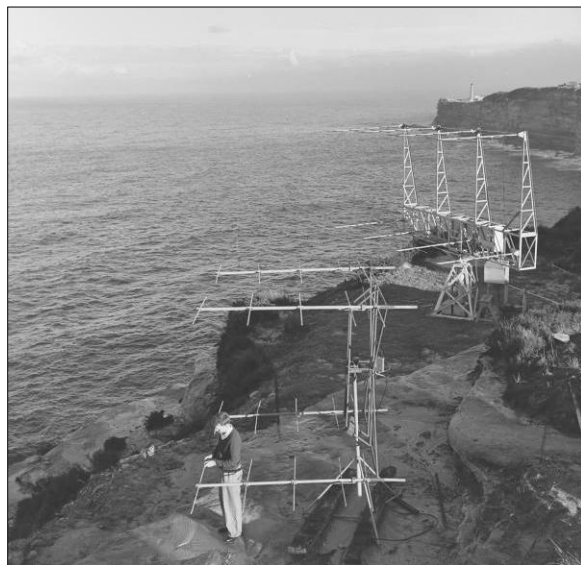
Figure 21: In the foreground is one of the two Yagi arrays of the azimuth interferometer (courtesy: CRAIA).
