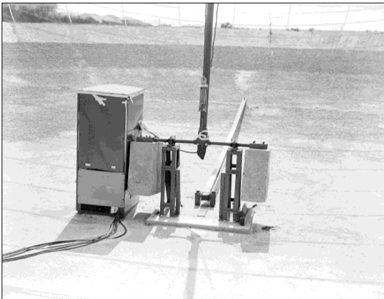
Figure 25: A close up of the water-tight box containing the second stage of the 400 MHz receiver located at the centre of the 80-ft HitGA (courtesy: CRAIA, B3150-5).
