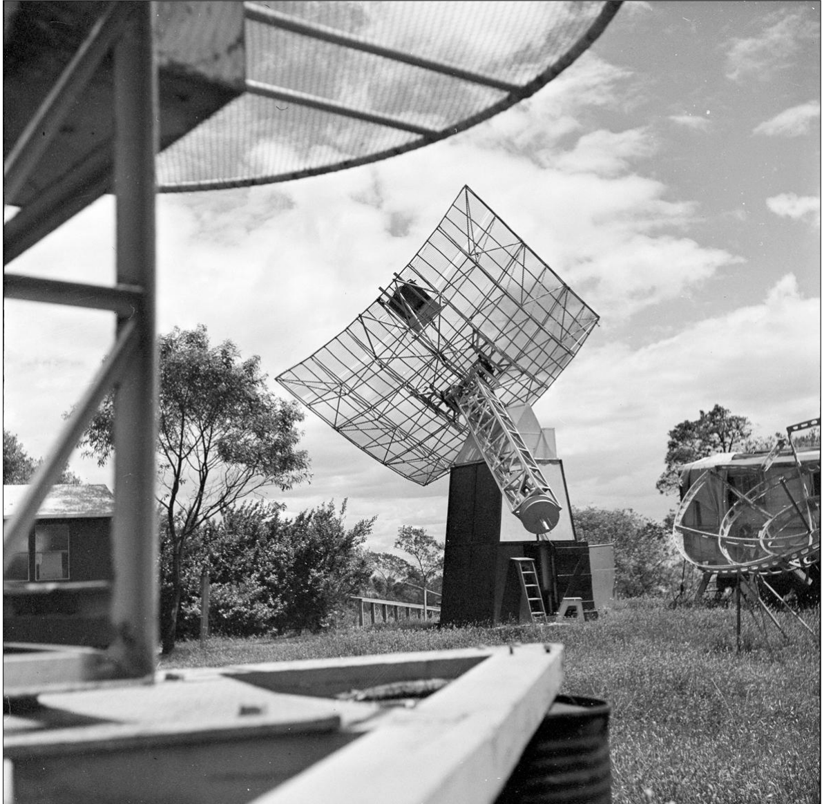
Figure 26: A view of the ex-Georges Heights antenna and on the extreme right the 10-ft U.S. radar antenna used by Piddington and Minnett for their 1,210 MHz all-sky survey (courtesy: CRAIA, B2639).
