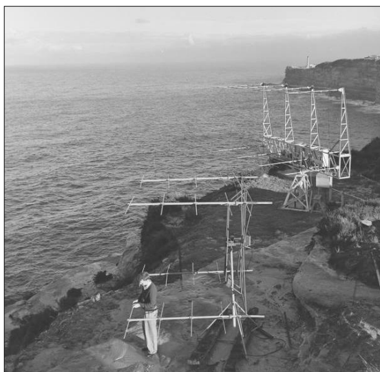
Figure 21: In the foreground is one of the two Yagi arrays of the azimuth interferometer (courtesy: CRAIA).
