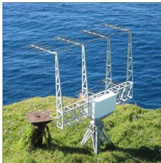
Figure 32: The rusting old antenna mount (on the left) and beside it the scaled-down replica of the 8-Yagi antenna (photograph: Harry Wendt).
