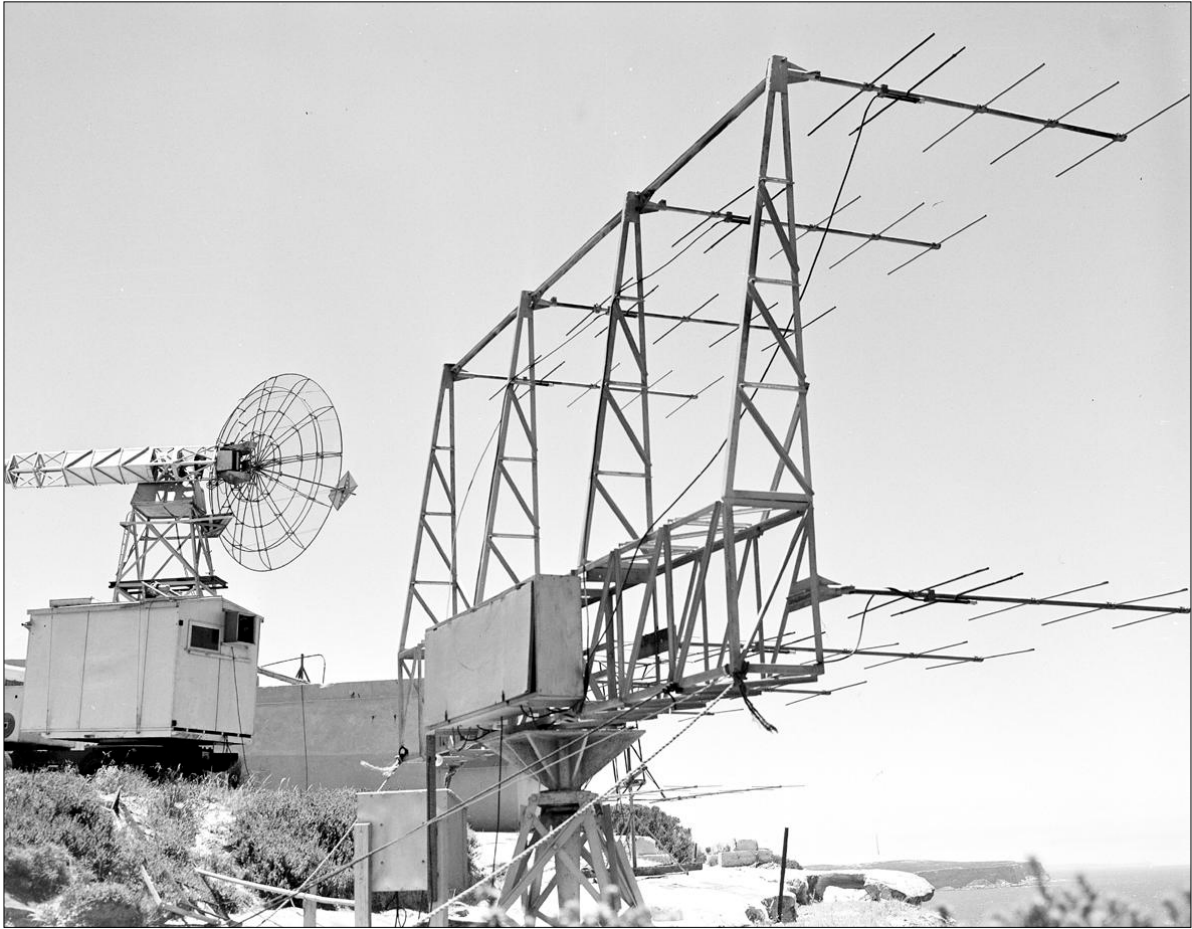
Figure 17: On the left is the 16-ft parabolic dish mounted on the gun-laying trailer and used as a sea interferometer, and in the foreground is the short-lived 8-Yagi array (courtesy: CRAIA B2650-6).
