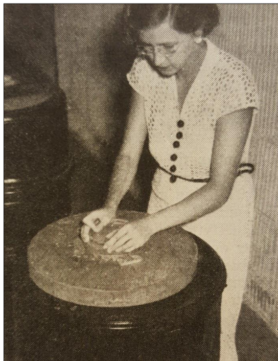
Figure 1: Mirror grinding (after Barton and Joseph, 1951: 171).
