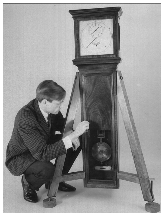
Figure 32: Shelton astronomical clock RS35, showing the replica tripod support (courtesy: the late Derek Howse).
