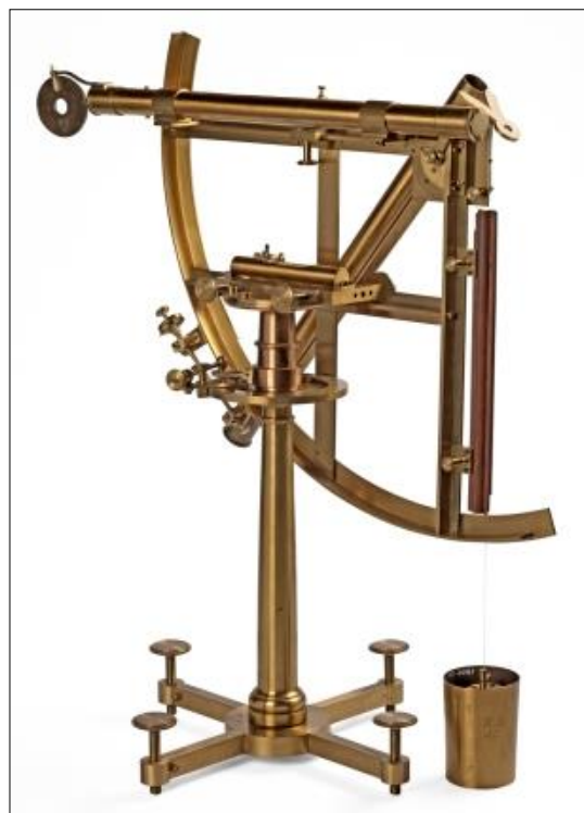
Figure 16: A 12-inch quadrant made by John Bird, which may have been on one of the British 1769 transit of Venus expeditions, but not necessarily the one to Tahiti (courtesy: The Royal Society, London).
