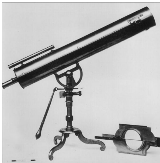
Figure 12: A Gregorian telescope by James Short, very similar if not identical to the ones that accompanied Cook and Green to Tahiti. At the bottom right is an object-glass micrometer that was used for measuring the angular separation of Venus from the limb of the Sun in the course of the transit (courtesy: The Royal Society, London).
