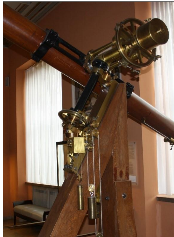
Figure 11: The Merz mounting and clock drive for the 19-cm refractor in Christiania, now on display in the Deutsches Museum in Munich with the 22-cm Merz refractor from Berlin Observatory that was used by Galle to discover Neptune (photograph: Bjørn Pettersen).
