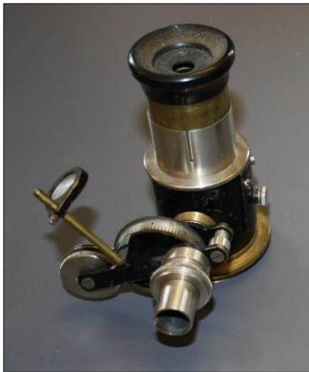
Figure 4: A ring micrometer (photograph: Bjørn Pettersen).
