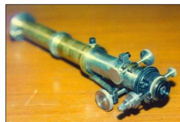
Figure 14: A Merz universal stellar spectroscope (photograph: Bjørn Pettersen).
