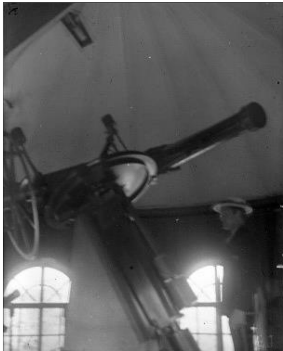
Figure 5: The Repsold-Merz equatorial refractor (unknown photographer/ courtesy: Norwegian Museum of Science and Technology).
