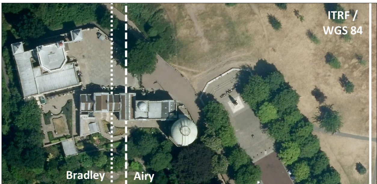
Figure 23: The Airy meridian (dashed line) adopted by the 1884 Meridian Conference and the actual ITRF zero meridian (solid line) (imagery copyright 2014 Google Maps. Infoterra Ltd & Bluesky).
