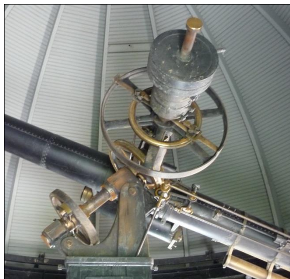
Figure 9: A close-up of the Drake University telescope's distinctive Warner & Swasey equatorial mounting (photograph: Deborah Kent).
