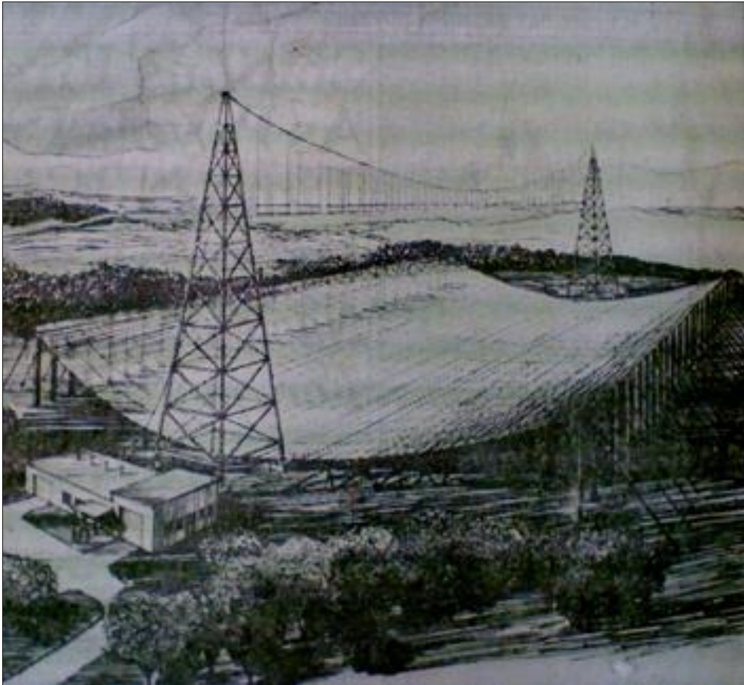
Figure 15: A concept drawing of a 500 ft (150 m) long cylindrical paraboloid to be located south of Ithaca. It was part of the publicity surrounding the establishment of the Center for Radiophysics and Space Research in November 1959 but was not built (courtesy: Cornell University Archives).
